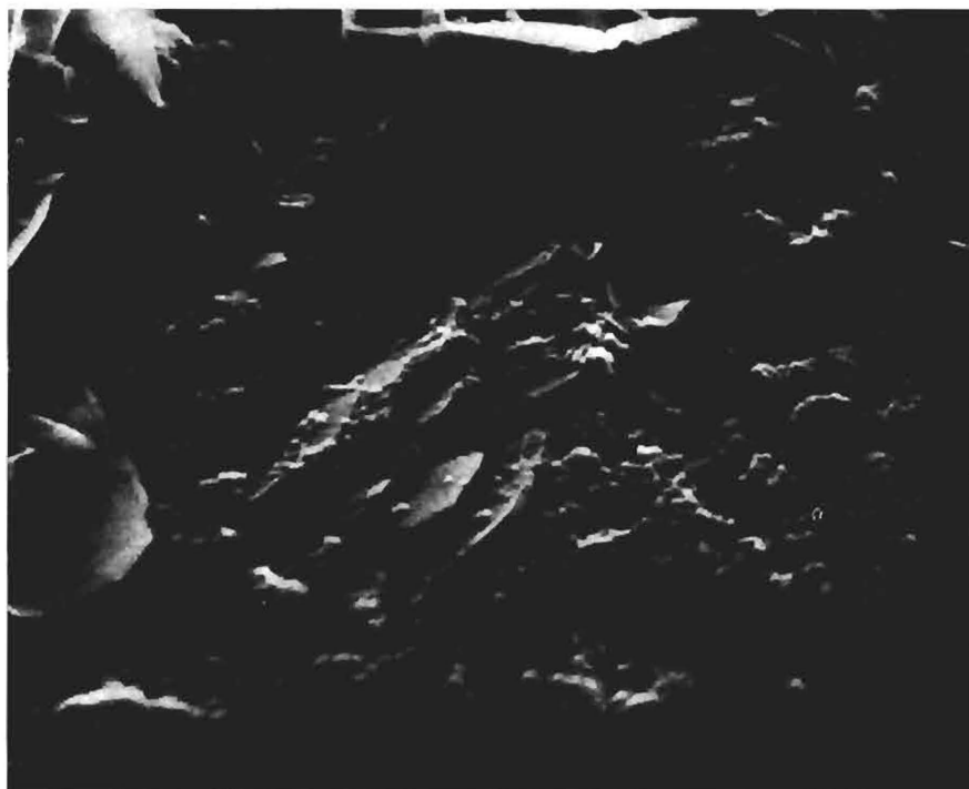
Figure 3. SEM Photomicrograph of Magnesium Hydroxide, or Brucite. The Magnification is 5,000\times ( 6\text{ mm}=1\text{ Micron} )
