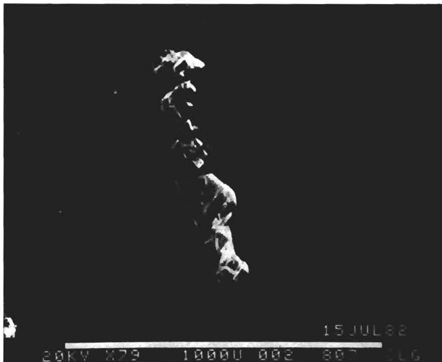
Figure 13. SEM Photomicrograph of Distorted Hemihydrate Formed from 2.75 × Gulf Seawater (Without Carbonate) Treated with \leq 1.25 mg/l Polycarboxylate under the Threshold Conditions of 4 Hours at 121°C (250°F) and an Initial pH of 9.00 \pm 0.05 . The Magnification is 79 \times (7.6 mm = 100 Microns)
