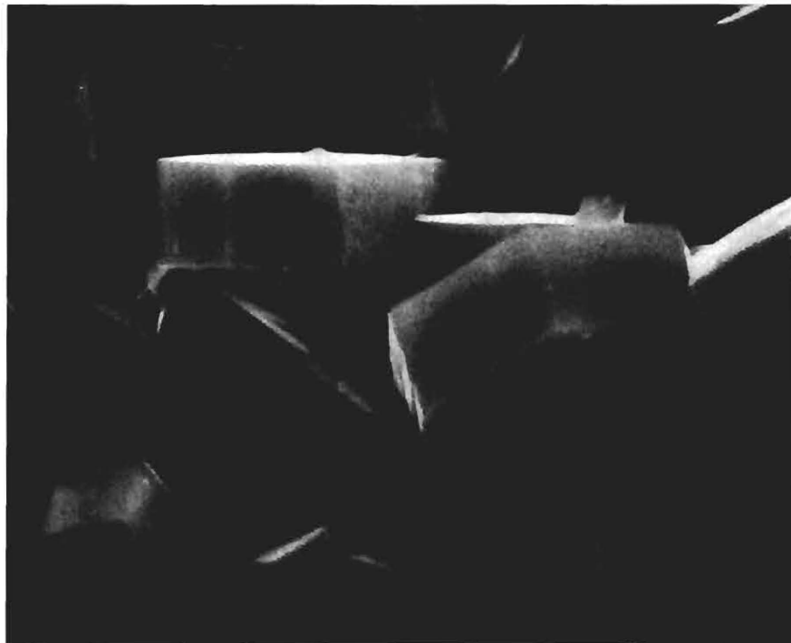
Figure 2. SEM Photomicrograph of Calcium Carbonate (Aragonite) Formed in 1.6 × Gulf Seawater at 116°C (240°F). The Magnification is 20,000 × (1 cm = 2 Microns)
