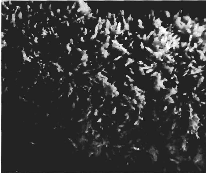
Figure 5. Zeiss Stereomicroscope Photograph of Uninhibited Calcium Sulfate Scale Formation on a SWSAS Tube ( 12\times ; 1\text{ cm}=1.2\text{ mm} )
