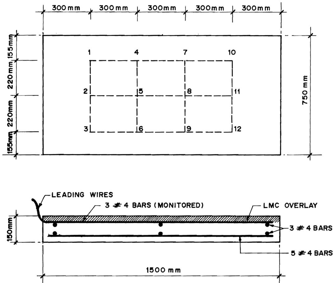
Figure 3. Reinforcement Detail and Points for Half-Cell Potential Measurements Corrosion Panel.
