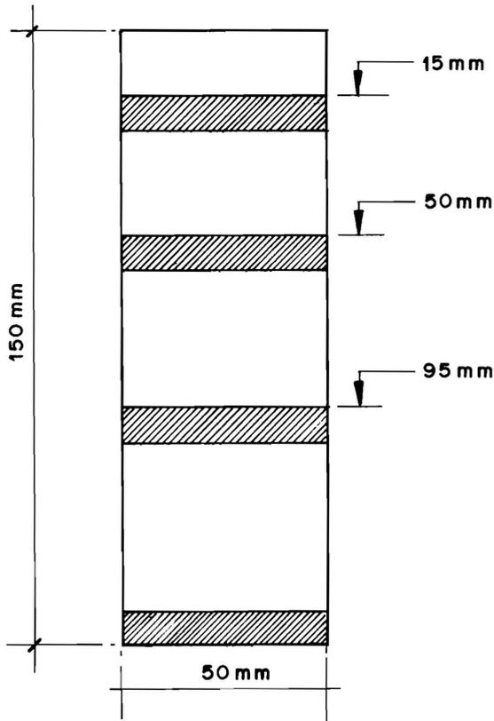
Figure 4. Core Sample Showing Slices 15 mm Thick Analyzed for Chloride Content.
