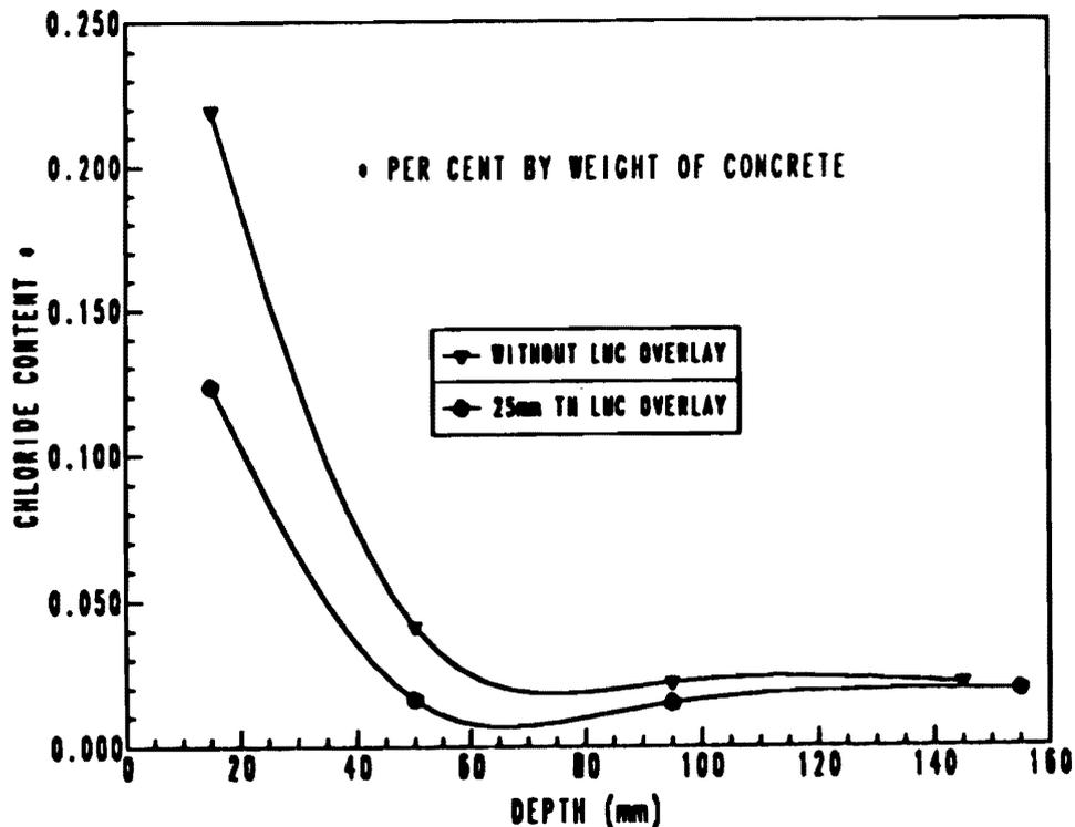
Figure 8. Chloride Content Variation versus Depth.
