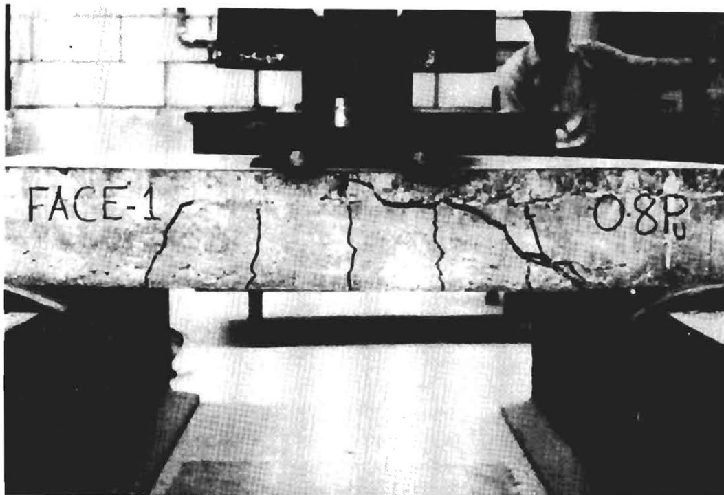
Figure 10. Failure of Composite Beam Under Cyclic Loading When Subjected to 80 Percent of Ultimate Static Load.
