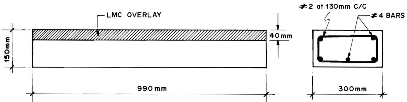
Figure 5. Dimensions and Reinforcement Details of Composite Beam Specimen.
