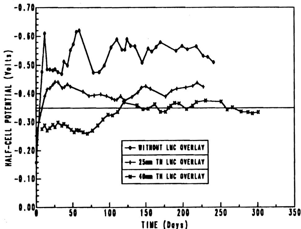
Figure 7. Half-Cell Potential Readings versus Time.
