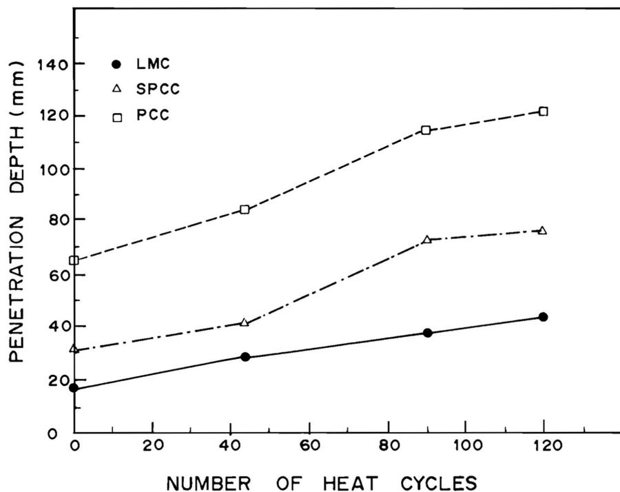
Figure 9. Depth of Water Penetration versus Heat Cycles.
