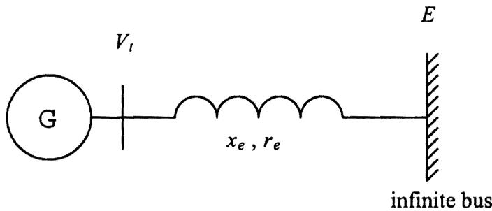
Figure 1. Single machine connected to an infinite bus.
