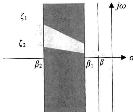
Figure 3. Vertical strip in the complex  $s$ -plane with bounds on the damping ratio.
