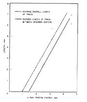
Figure 3. Track dimension versus X-ray photon energy.
