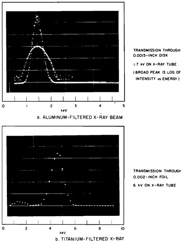
Figure 1. Intensity of filtered X-ray beams versus X-ray photon energy.
