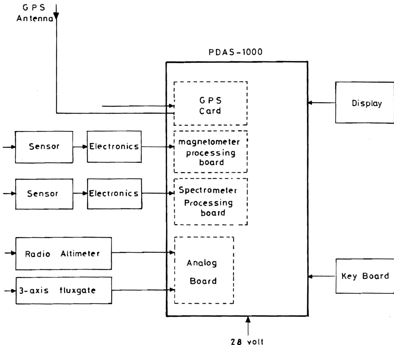
Figure 1. Block diagram for the PDAS-1000 Egyptian Airborne Geophysical Survey System (EAGSS).
