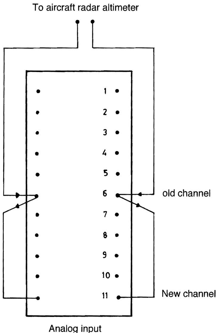
Figure 14. Rear panel of the analog board of the PDAS-1000 of the EAGSS, with the new altitude channel recording from 0.0–2500 ft (0–762.0 m).
