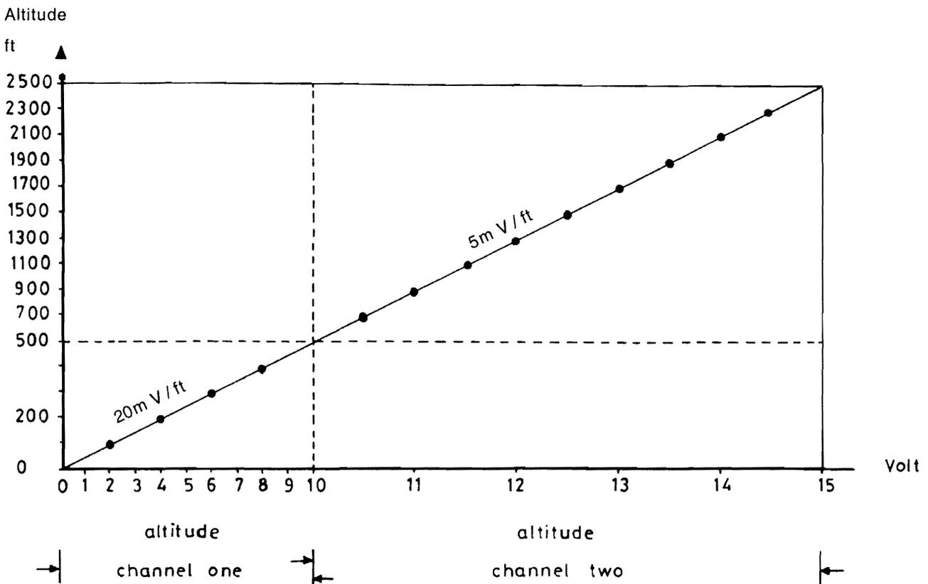
Figure 3. The two channels for altitude recording (0-500 ft and 0-2500 ft) used for the control design of the PDAS-1000 of the EAGSS.
