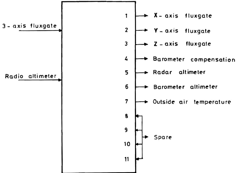
Figure 2. Rear panel of the analog board of the PDAS-1000 of the Egyptian Airborne Geophysical Survey System (EAGSS).
