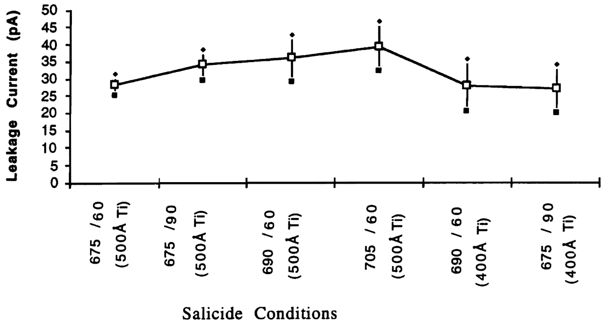
Figure 9. The effect of salicide first RTP anneal step (temperature/time) and titanium thickness on the leakage current of area intensive P+/N diodes.
