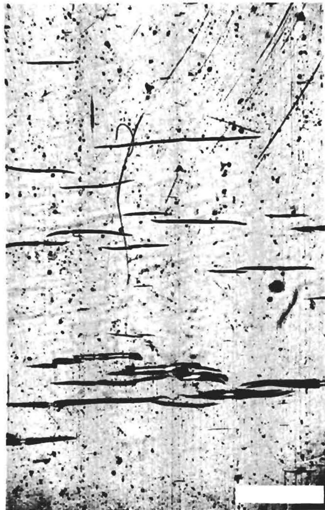
Figure 4. Photomicrograph of a Polyamide-6 Film After Two-Months Weathering Under Stress on Glass Cylinder. The cracks are aligned perpendicularly to the stress direction. Bar is 5 mm.
