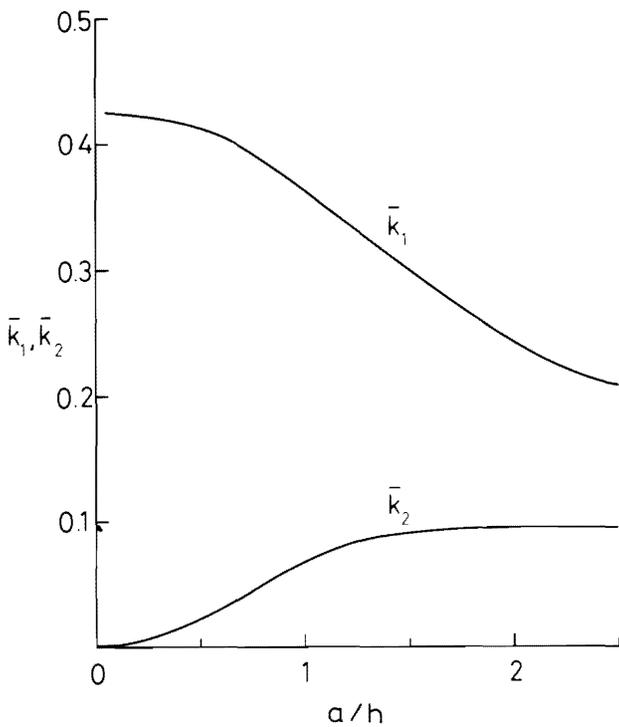
Figure 4. Stress Intensity Factors at the Corners of the Rigid Block.
