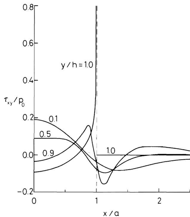
Figure 6. Shear Stress Distributions when  $a = h$ .
