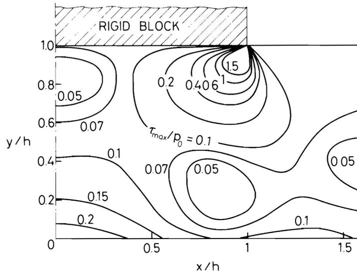
Figure 9. Maximum Shear Stress Contours when  $a = h$ .
