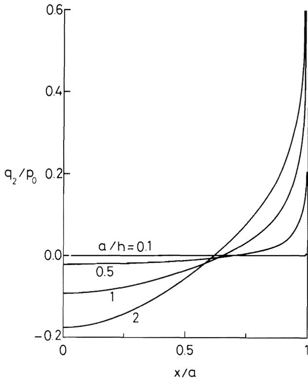
Figure 3. Shear Stress Between the Layer and the Rigid Block.
