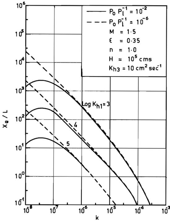
Figure 6. Influence of Porous Parameter  $P_0 P_l^{-1}$  on Relative Damping-Length
