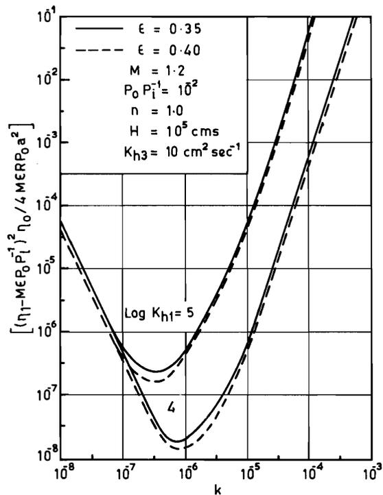
Figure 3. Influence of Porosity on Frequency of Internal Waves
