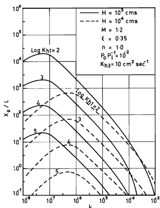
Figure 5. Influence of Thickness of Porous Layer on Relative Damping-Length
