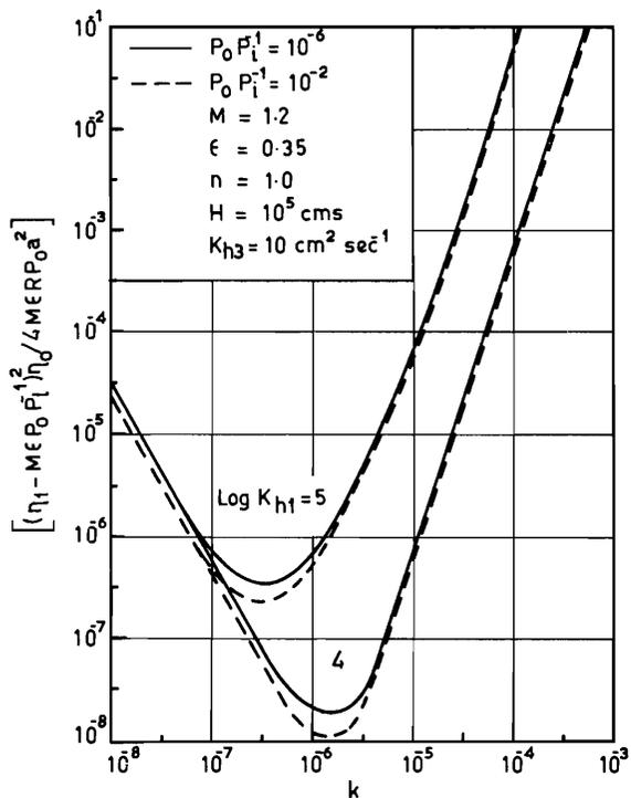
Figure 2. Influence of  $P_o P_l^{-1}$  on Frequency of Internal Waves
