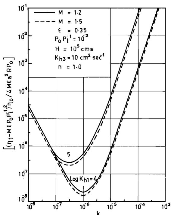
Figure 4. Influence of Ratio,  $M$ , of Heat Capacities of Pores and Fluid on Frequency of Internal Waves
