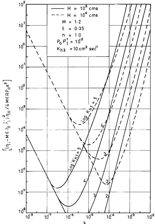
Figure 1. Influence of Thickness of Porous Layer on Frequency of Internal Waves
