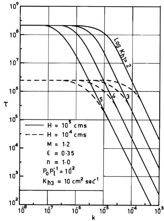
Figure 7. Influence of Thickness of Porous Layer on Damping-Rate
