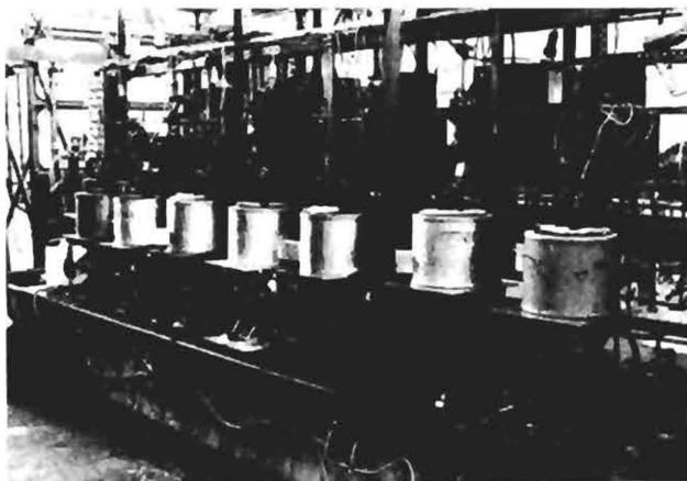
Figure 7. Screening Test Unit with Isothermic Integral Reactors
