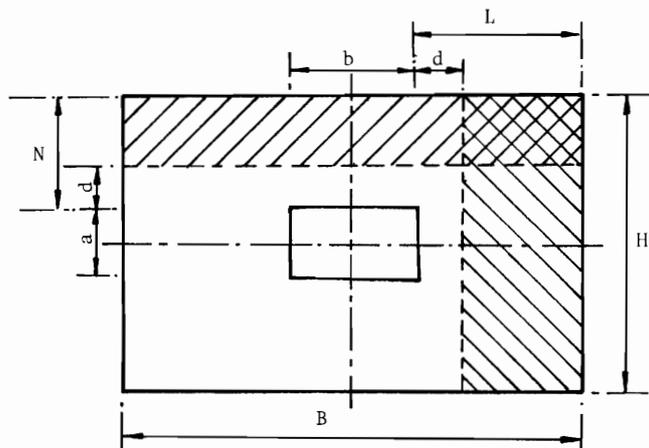
Figure 4. Critical Sections for Beam Actions
