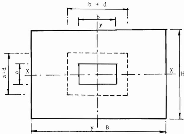
Figure 3. Critical Sections for Two-way Slab Action
