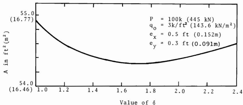
Figure 2. Area of Footing versus  $\delta$
