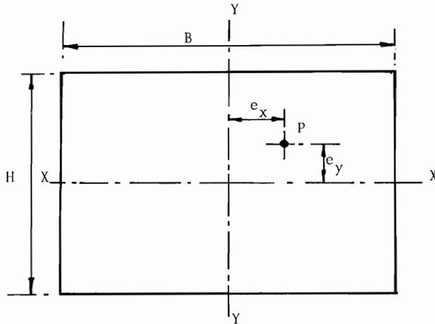
Figure 1. A Typical Footing under Eccentric Load
