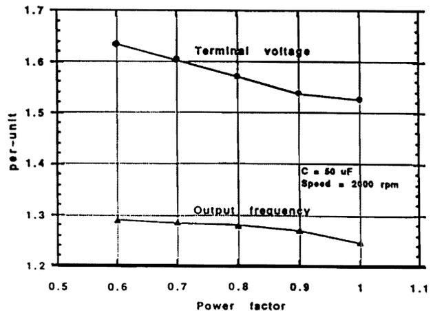
Figure 6. Steady State Performance of 1 kW Generator at Different Power Factors for Load of 200  $\Omega$ .
