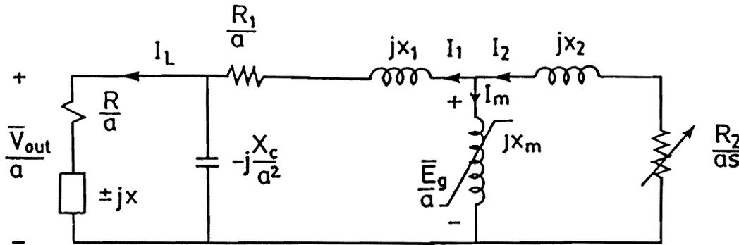
Figure 1. The Steady-State Equivalent Circuit of an Induction Generator.
