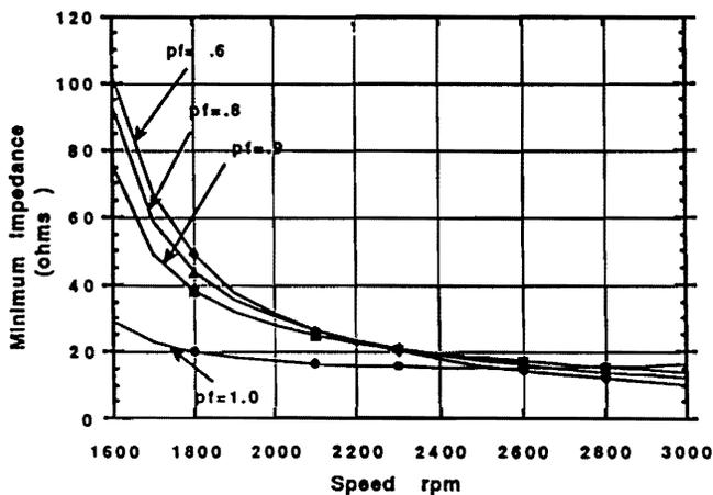
Figure 5. Variation of Minimum Load Impedance with Speed at Different Lagging Power Factors. For 10 hp machine with capacitance of 120  $\mu$ F.
