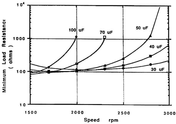
Figure 3. Minimum Load Resistance for 1 kW Machine.
