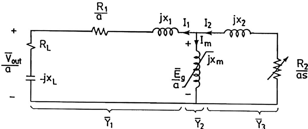
Figure 2. A Simplified Equivalent Circuit of an Induction Generator.
