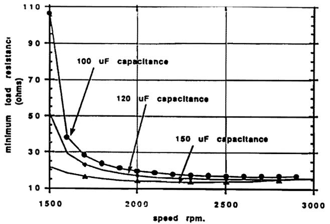
Figure 4. Minimum Load Resistance for 10 hp Machine for Pure Resistive Load.
