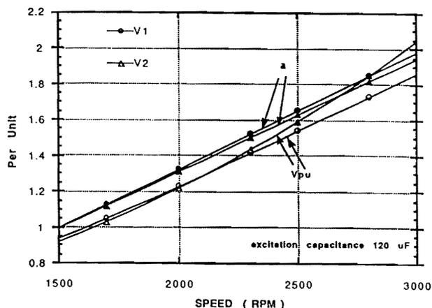
Figure 8. Steady State Performance of 10 hp Induction Generator for a Pure Resistive Load of 200 Ω.
