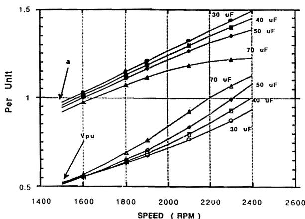
Figure 7. Steady State Performance of 5 hp Induction Generator for a 200 Ω Resistive Load.
