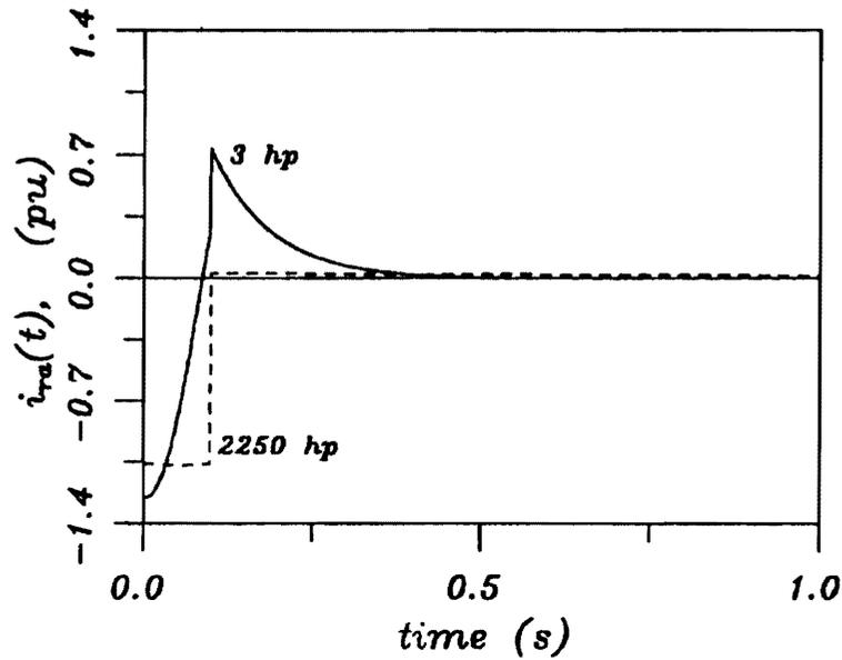
Figure 3. Phase a rotor Currents of the Two Machines Before and After they were Disconnected from the System.
