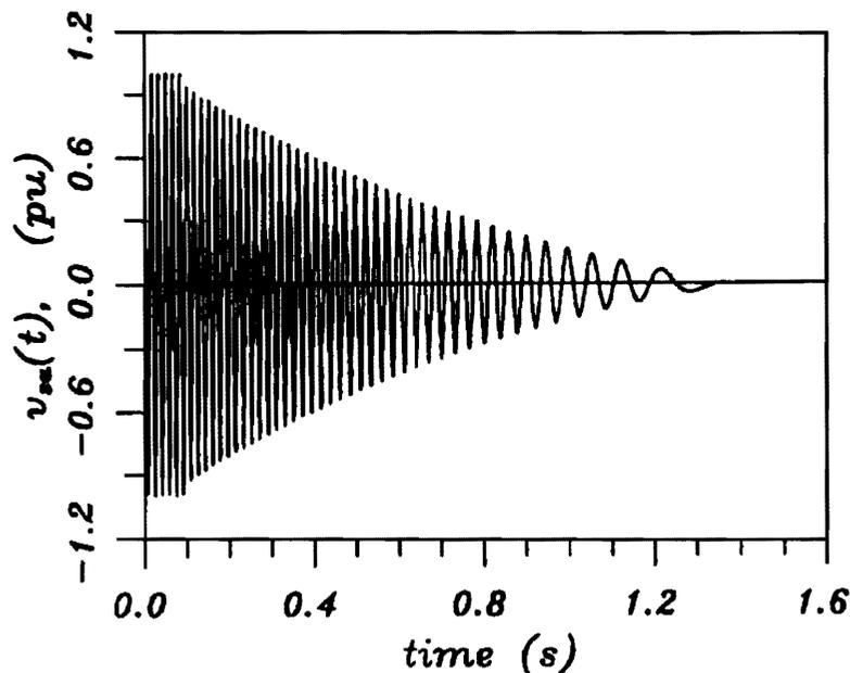
Figure 1. Phase a Stator Voltage of the 2250 hp Machine Before and After it was Disconnected from the System.
