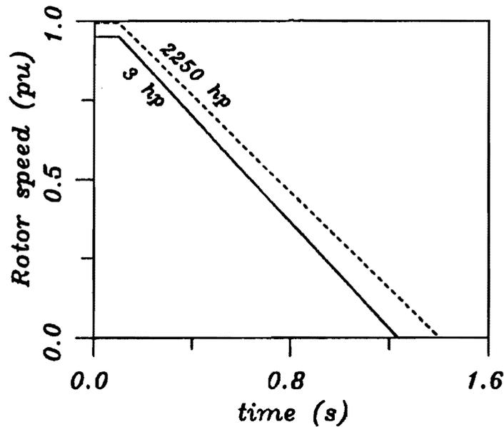
Figure 4. Rotor Speeds of the Two Machines Before and After they were Disconnected from the System.
