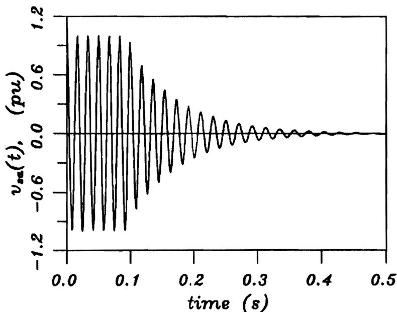
Figure 2. Phase a Stator Voltage of the 3 hp Machine Before and After it was Disconnected from the System.
