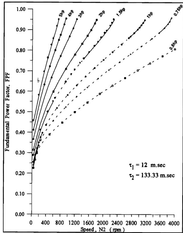
Figure 11. Supply fundamental power factor versus speed  $N_2$  of the system operation at different values of horsepower levels of motor 2, at  $N_1=2500$  rpm.
