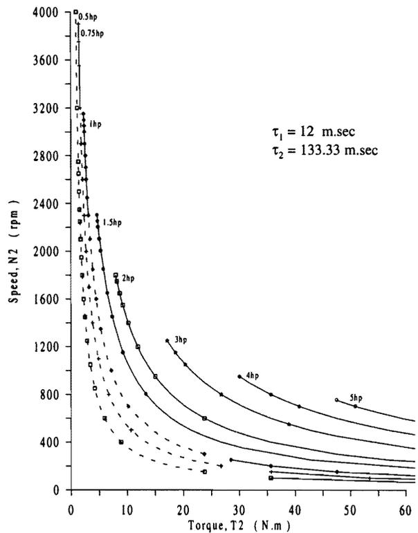
Figure 7. Torque-speed characteristics ( N2 versus T2 ) of the system operation at different values of horsepower levels of motor 2, at N1 = 1500 rpm.
