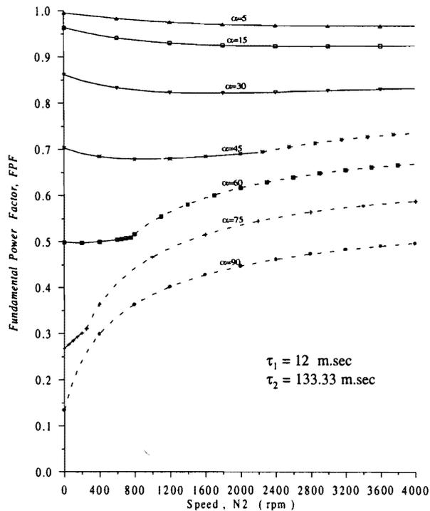
Figure 9. Supply fundamental power factor versus speed N2 of the system operation at different values of firing angles, at N1 = 1000 rpm.
