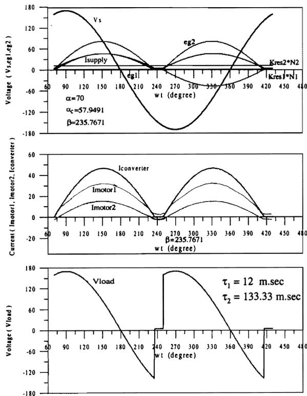
Figure 4. Current and voltage waveforms of the system operation in discontinuous converter current mode at  $N1=500$  rpm,  $N2=1500$  rpm, and  $\alpha = 70$  deg.
