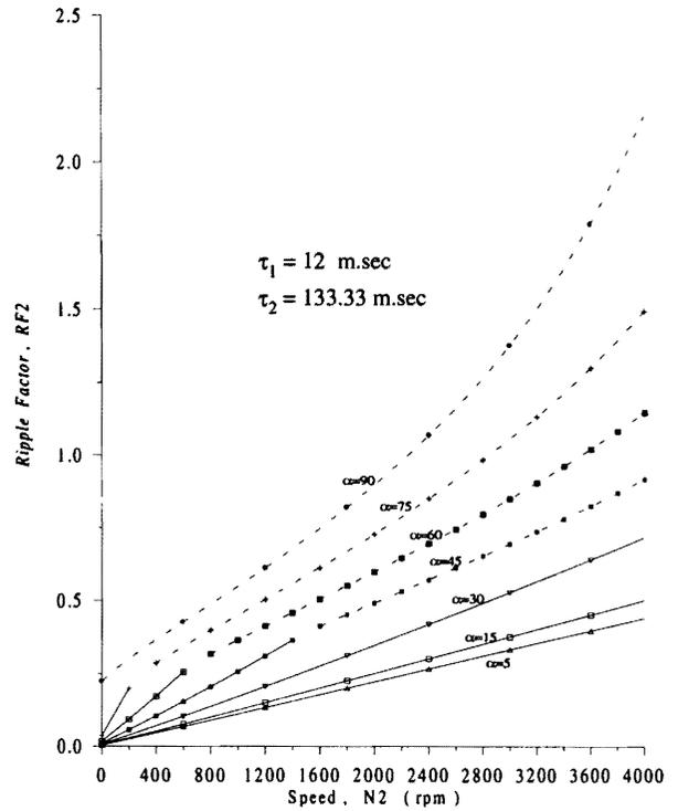
Figure 17. Current ripple factor of motor two versus speed N2 of the system operation at different values of firing angles, at N1=1500 rpm.
