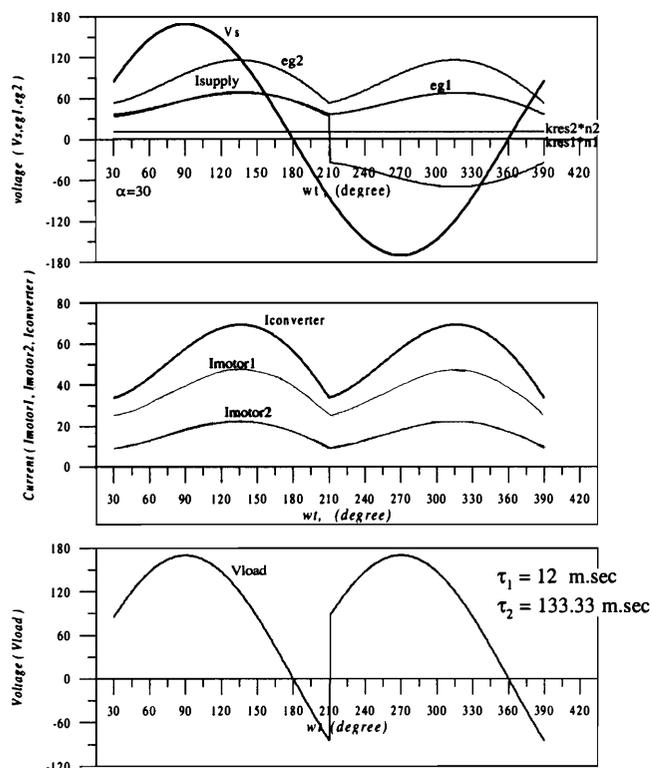
Figure 3a. Current and voltage waveforms of the system operation in continuous converter current mode at N1=500 rpm, N2=1500 rpm, and  $\alpha = 30\text{deg}$ .
