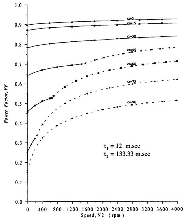
Figure 8. Supply power factor versus speed N2 of the system operation at different values of firing angles, at N1=1500 rpm.
