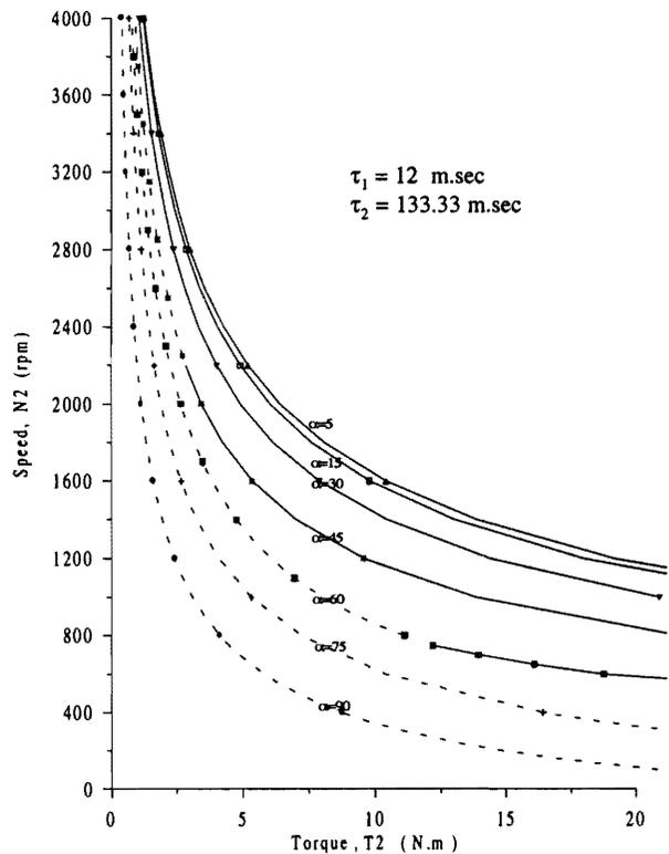
Figure 5. Torque-speed characteristics ( $N2$  versus  $T2$ ) of the system operation at different values of firing angles at  $N1= 1000$  rpm.
