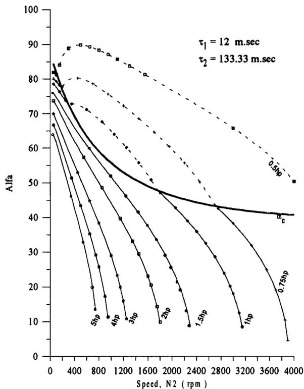
Figure 6. Firing angle versus speed N2 of the system operation at different values of horsepower levels of motor 2, at N1=1000 rpm.
