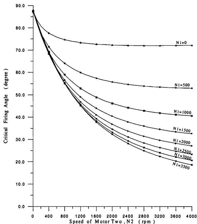
Figure 2. The critical firing angle versus speed N2 for different values of speed N1.
