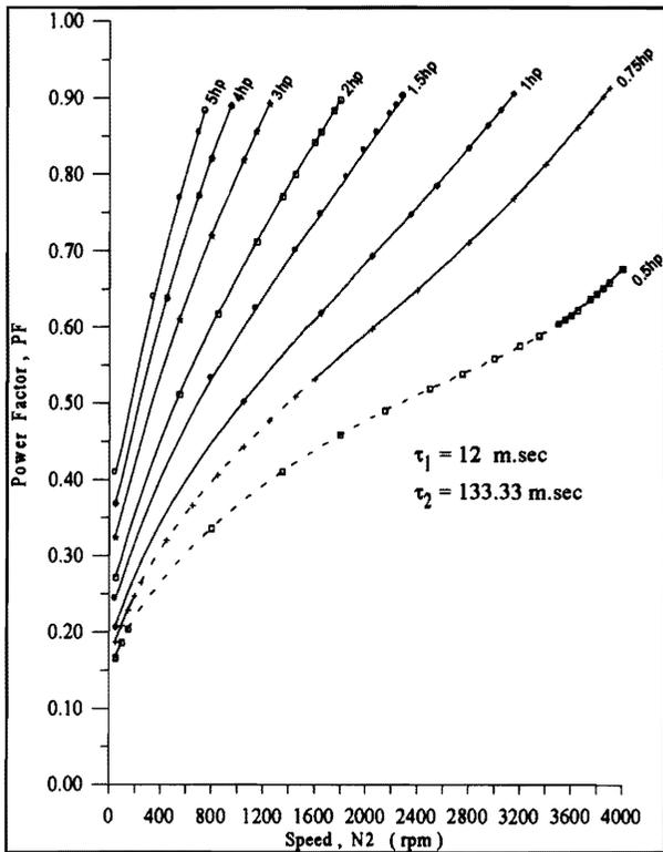
Figure 10. Supply power factor versus speed  $N_2$  of the system operation at different values of horsepower levels of motor 2, at  $N_1=500$  rpm.
