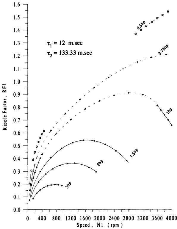
Figure 14. Current ripple factor of motor one versus speed N1 of the system operation at different values of horsepower levels of motor 1, at N2=1500 rpm.
