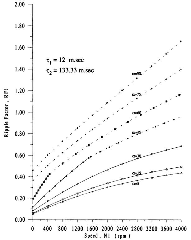
Figure 15. Current ripple factor of motor one versus speed N1 of the system operation at different values of firing angles, at N2=1500 rpm.
