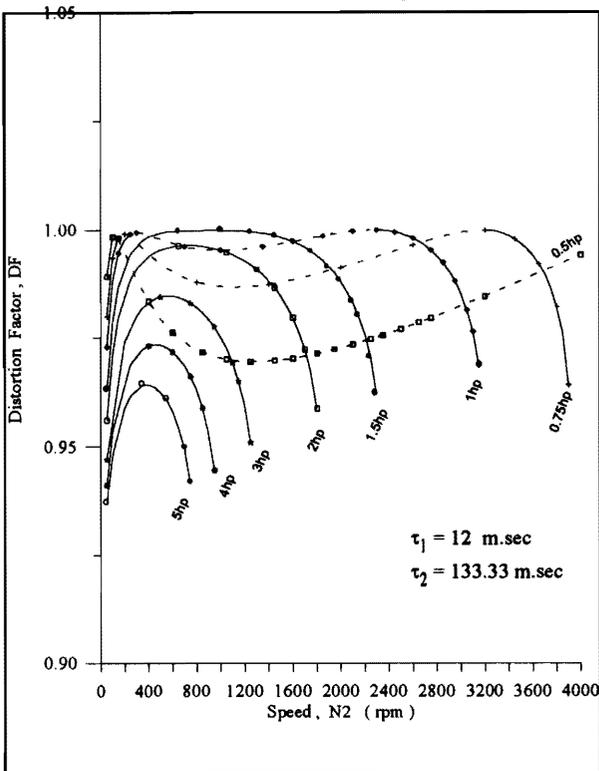
Figure 12. Distortion factor versus speed  $N_2$  of the system operation at different values of horsepower levels of motor 2, at  $N_1=1500$  rpm.
