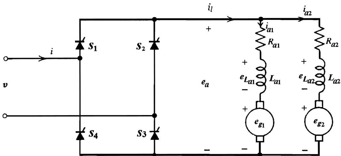
Figure 1. Terminal voltage control of two DC series motors by a single phase full-converter.
