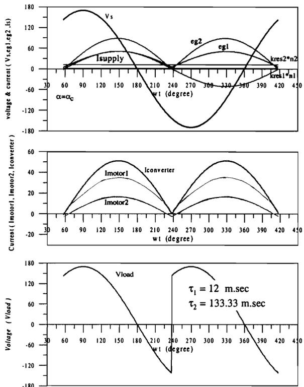
Figure 3b. Current and voltage waveforms of the system operation in continuous converter current mode at N1=500 rpm, N2=1500 rpm, and  $\alpha = \alpha_c = 57.949\text{ deg}$ .
