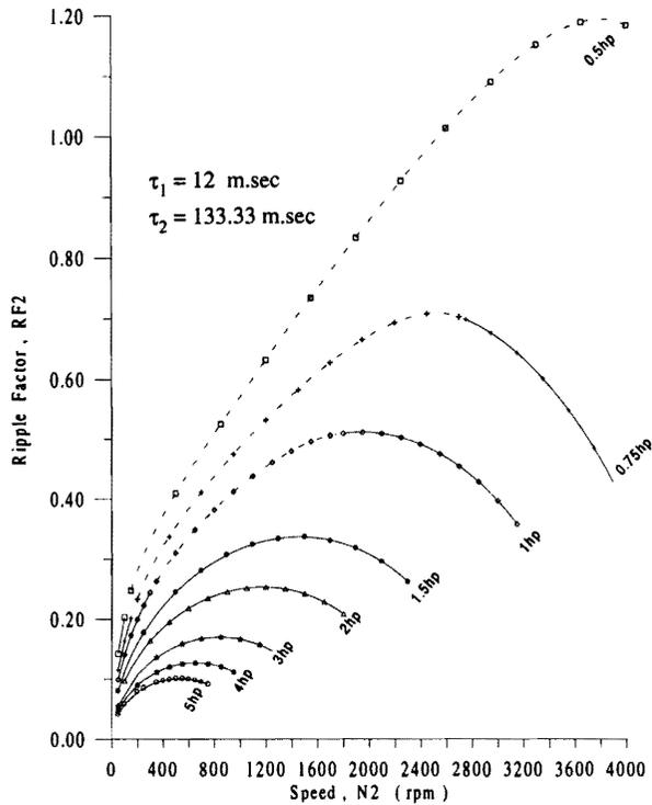
Figure 16. Current ripple factor of motor two versus speed N2 of the system operation at different values of horsepower levels of motor 2, at N1=1000 rpm.
