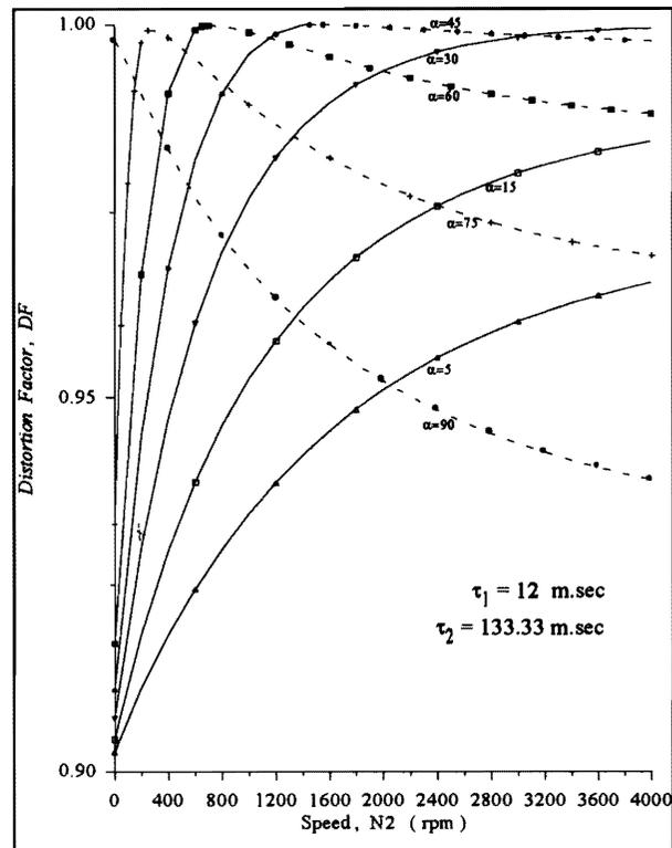
Figure 13. Distortion factor versus speed  $N_2$  of the system operation at different values of firing angles, at  $N_1=1500$  rpm.
