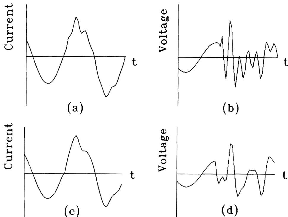
Figure 2. Unfiltered Optimized Waveforms for FS and PM Relays. (a), (b): FS Relay; (c), (d): PM Relay.
