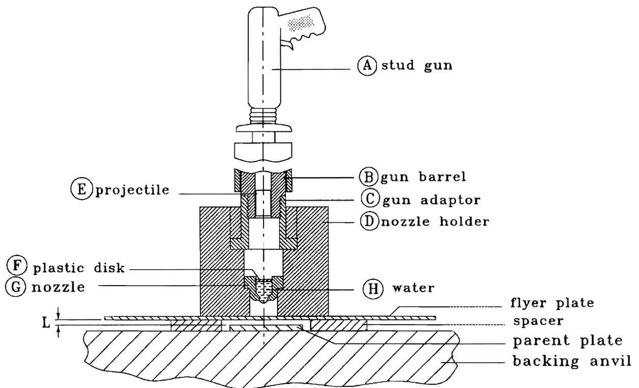
Figure 1. Schematic Representation of the Impact of a Jet of Water.
