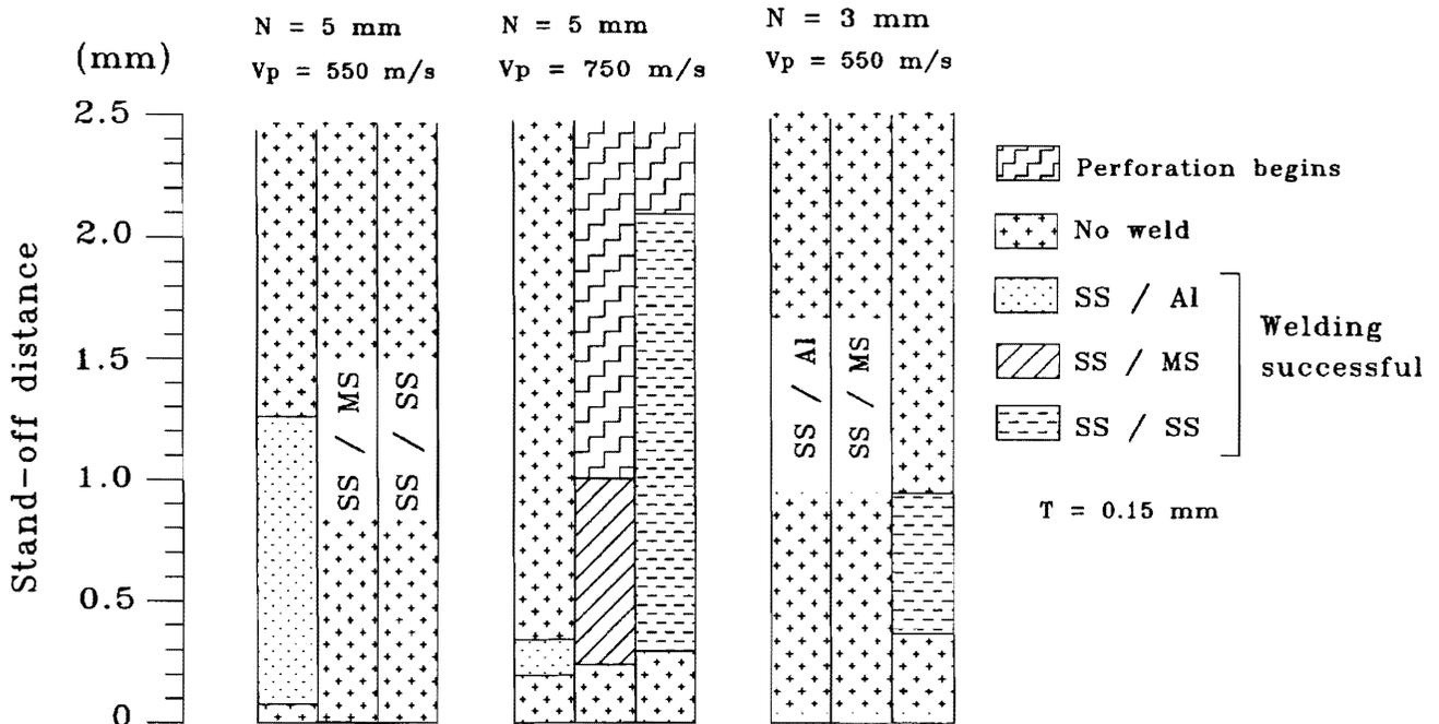
Figure 4. Results of Welding Experiments with MS Flyer Plates.
