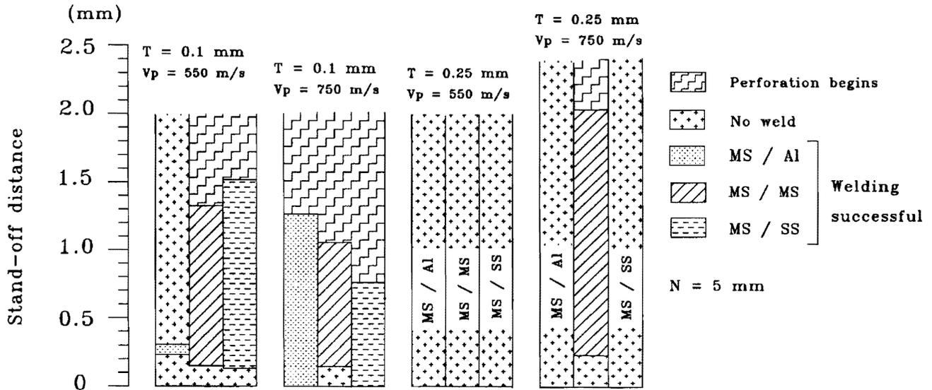
Figure 3. Results of Welding Experiments with Al Flyer Plates.
