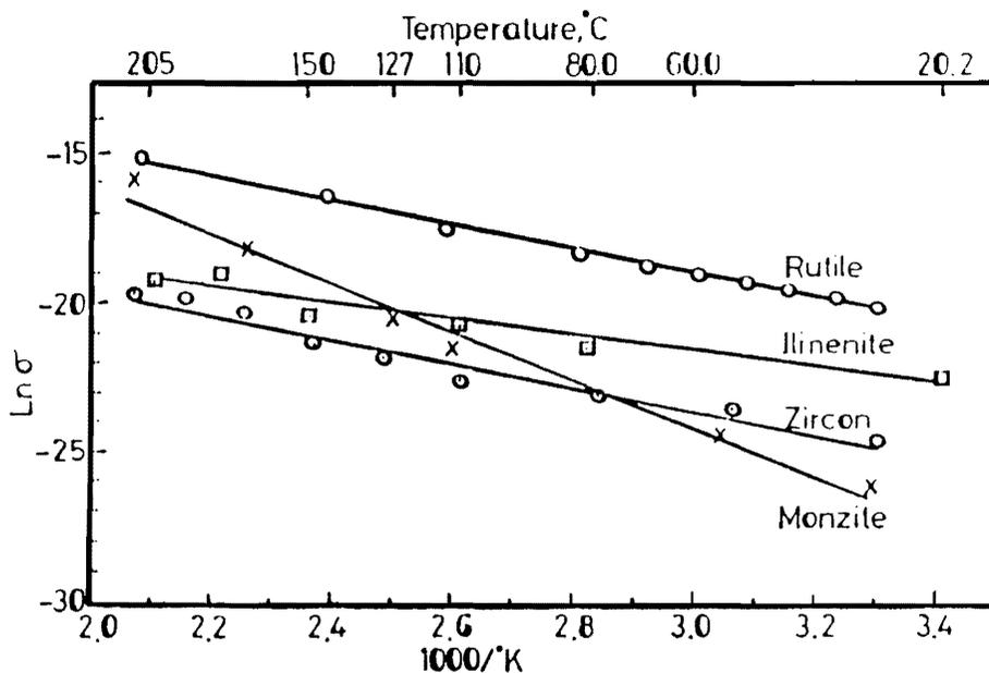
Figure 7. Temperature Dependence of Conductivity.
