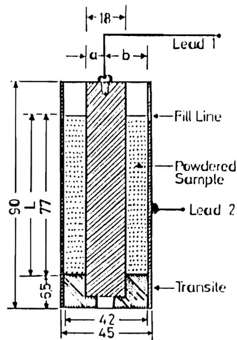
Figure 1. Detail of the Conductivity Cell. Dimensions are in Millimeters.
