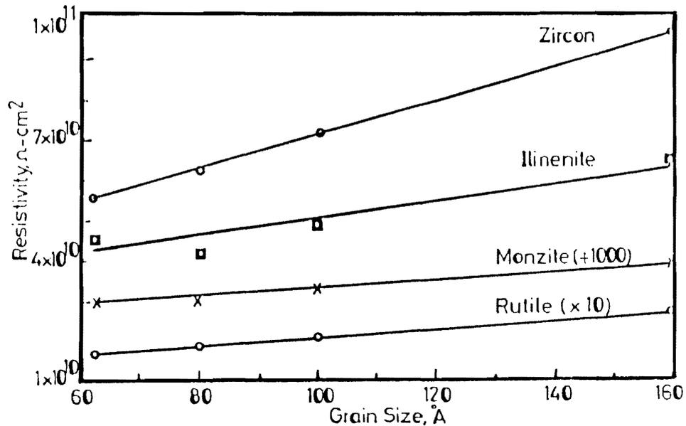
Figure 8. Grain Size Dependence of Conductivity.
