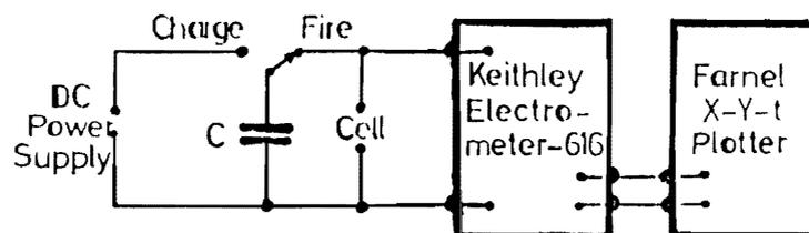
Figure 2. Schematic Diagram of the Discharge Circuit.
