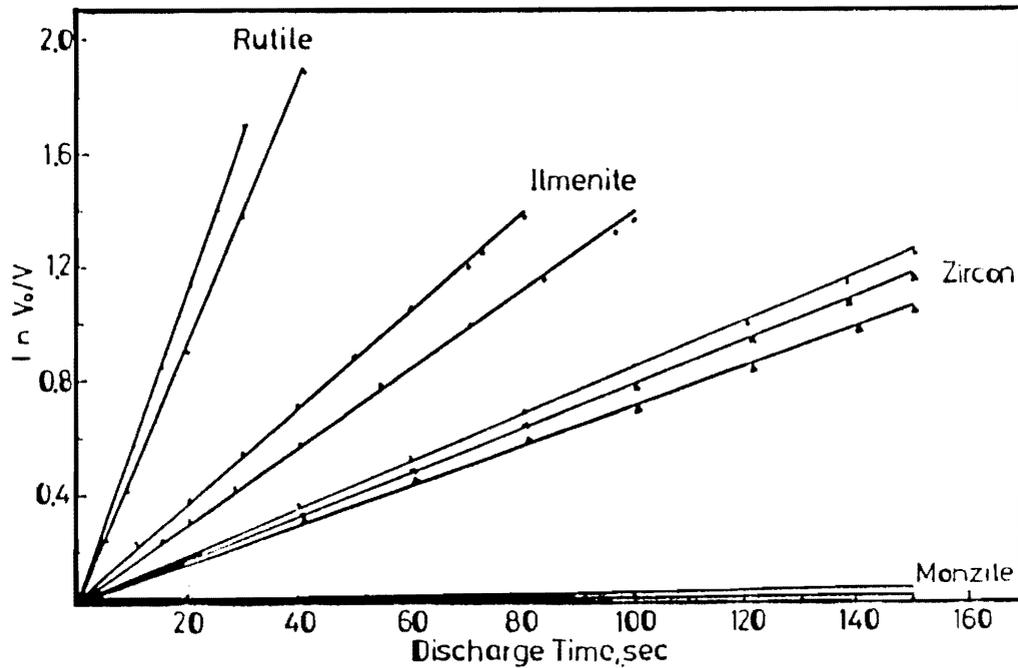
Figure 4.  $\ln(V_0/V)$  Versus Discharge Time for the Investigated Minerals.
