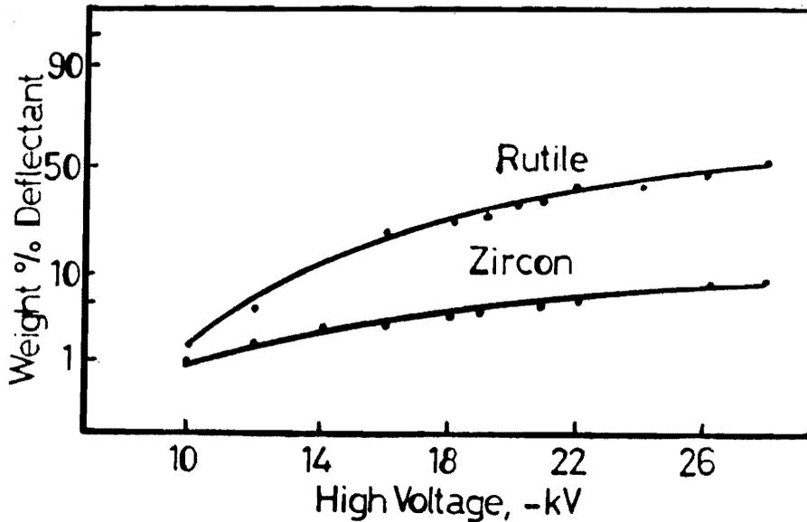
Figure 5. Effect of Voltage on the Electrostatic Deflection of Zircon and Rutile.
