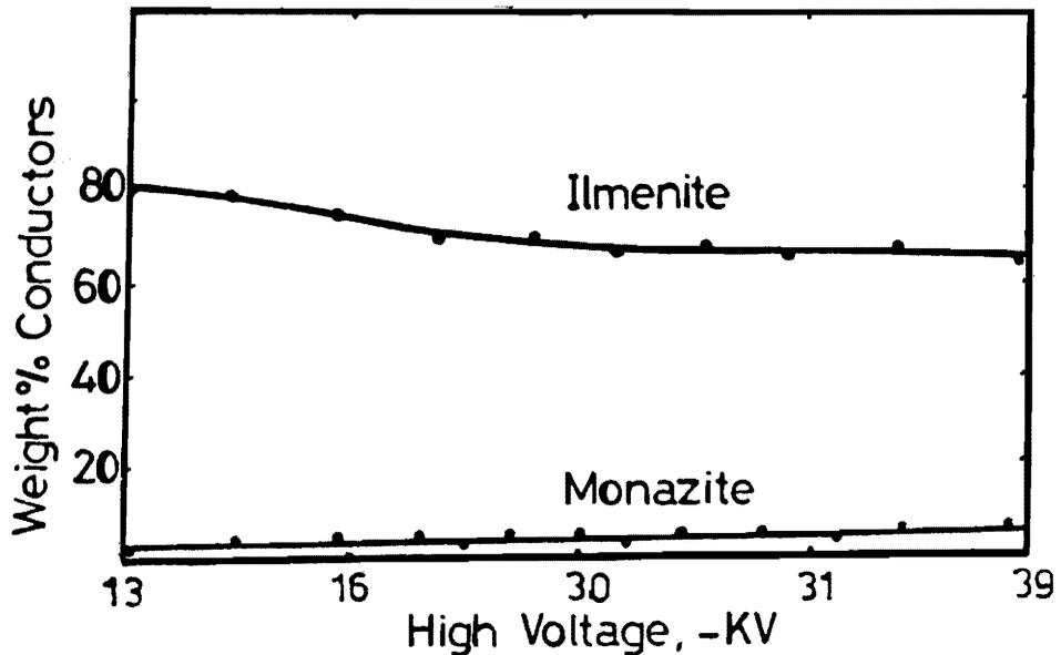
Figure 6. Effect of Voltage on the Electrostatic Deflection of Ilmenite and Monazite.
