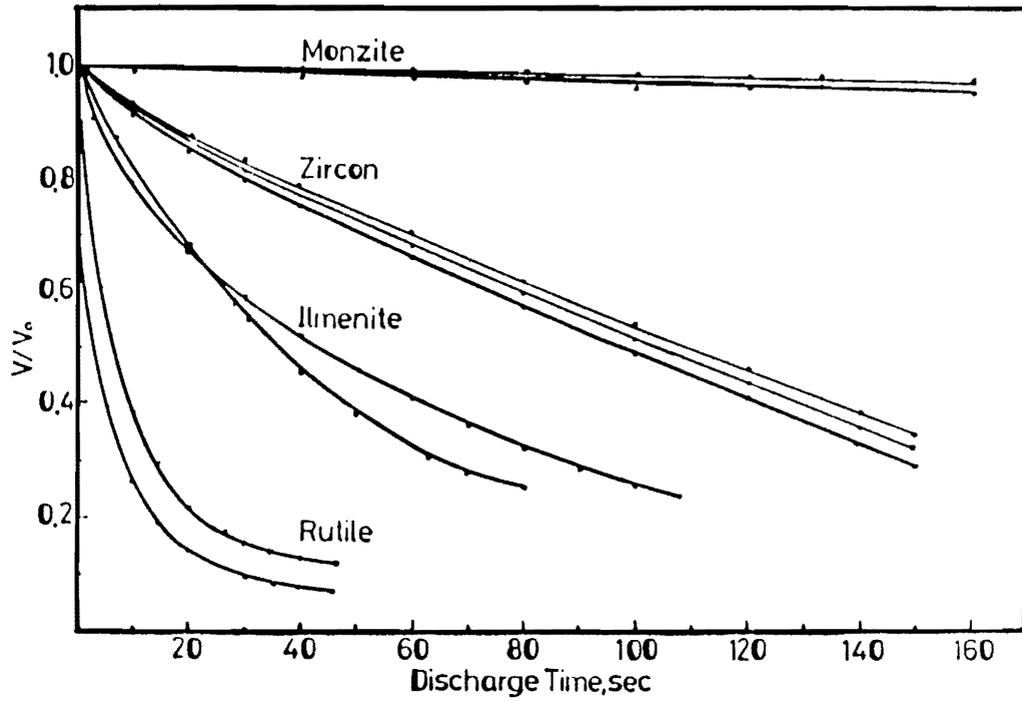
Figure 3. Discharge Curves for Monazite, Zircon, Ilmenite and Rutile. Samples are Collected from Different Locations.
