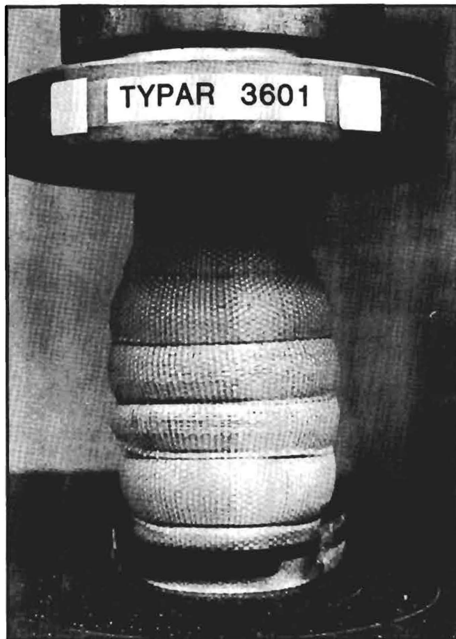
Figure 2. Deformed Shape of Encapsulated/Internally Reinforced Sand Tests in Uniaxial Compression.
