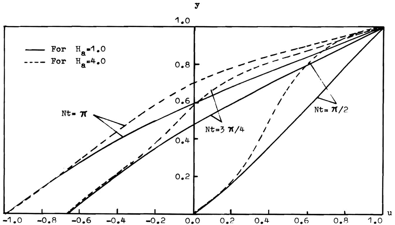
Figure 2. Velocity Profiles Plotted Against  $y$  for  $\alpha=-1.0$ ,  $R_e=2$ , and  $\beta=1$ .
