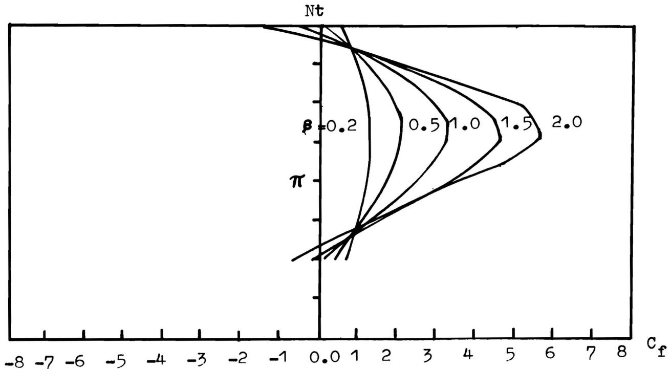
Figure 5. Coefficients of Skin Friction Plotted Against  $Nt$  where  $\alpha = -1$ ,  $H_a = 1$ ,  $\beta = 0.2, 0.5, 1, 1.5, 2$ .
