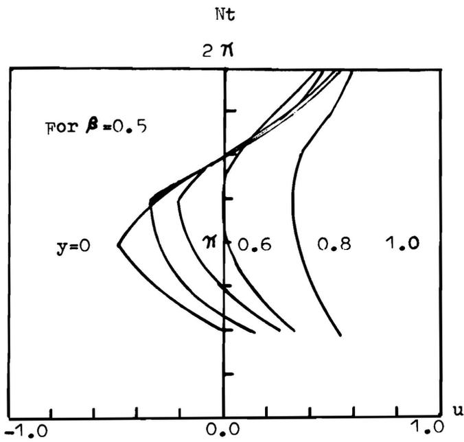
Figure 3. Velocity Profiles Plotted Against  $Nt$  for  $\alpha = -1.0$ ,  $R_e = 2$ , and  $\beta = 0.5$ .
