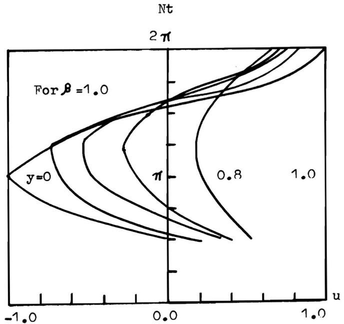
Figure 4. Velocity Profiles Plotted Against  $Nt$  for  $\alpha = -1.0$ ,  $R_e = 2$ , and  $\beta = 1.0$ .
