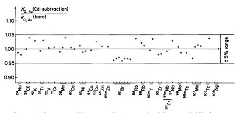
Figure 1. Comparison of Experimentally Determined and Recommended K<sub>0</sub>-factors
