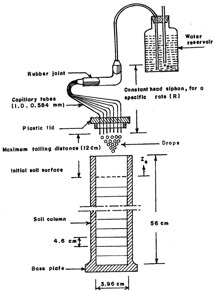
FIG. 2. Schematic diagram of the experimental set up, showing the sectionized soil column under the sprinkler simulator.  $Z_e$  is the absolute expansion above the initial soil surface.
