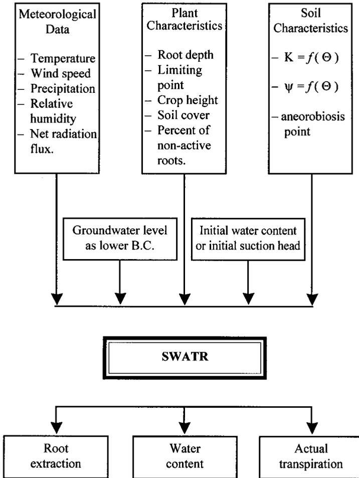
FIG. 1. Input-output description for the SWATR model.
