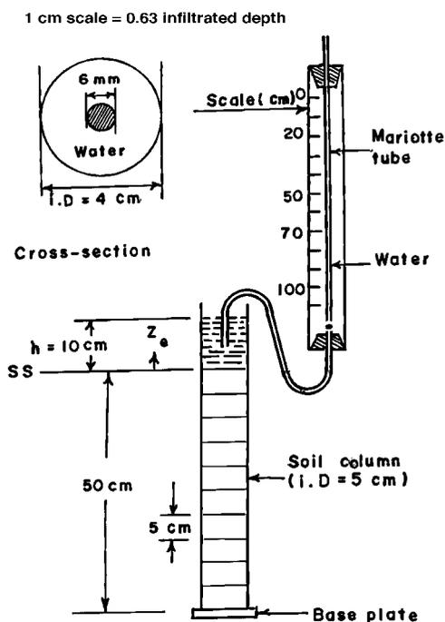
FIG. 1. Schematic diagram of the ponded infiltration experiment.  $Z_e$  is the absolute expansion above the initial soil surfaces (SS).
