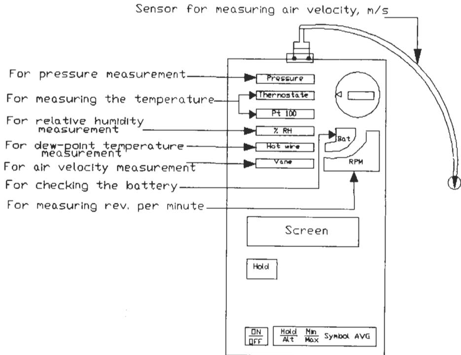
FIG. 3. Solomat; air velocity, relative humidity, and temperature meter.
