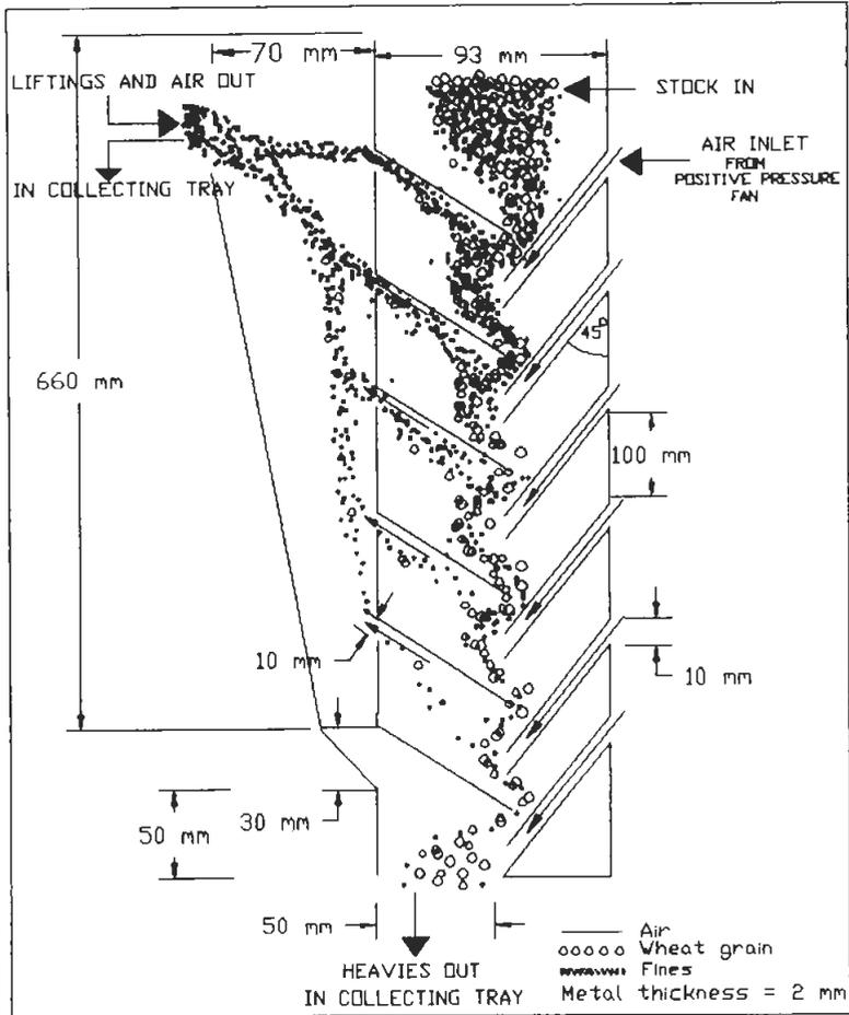
FIG. 1. Cross section of miniaspirator.
