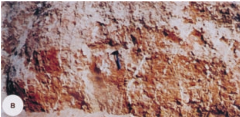
PLATE 1b. Slightly fissile, brown to brownish white, silty to sandy clay of Ubhur Formation dissected by oriented fractures filled with carbonate and gypsum. Siliceous small nodules are also interbedded, locality UB1.
