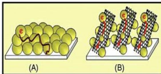
**Scheme 1. Electron transport across nanostructured semiconductor films: (A) in the absence, and (B) in the presence of nanotube support architecture <sup>[22]</sup>.**
