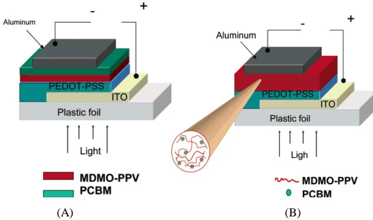
Fig. 5: (A) Bilayer configuration in organic solar cells <sup>[44]</sup> .(B) Bulk heterojunction configuration in organic solar cells<sup>[44]</sup>.
