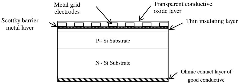
**Fig. 1. Schematic physical structure of a typical Silicon Schottky junction solar cell. (Sketch adapted from [9, 10]).**
