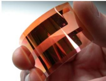
Fig. 6. Polymer-Fullerene Bulk Heterojunction Photovoltaic cell <sup>[46]</sup>.
