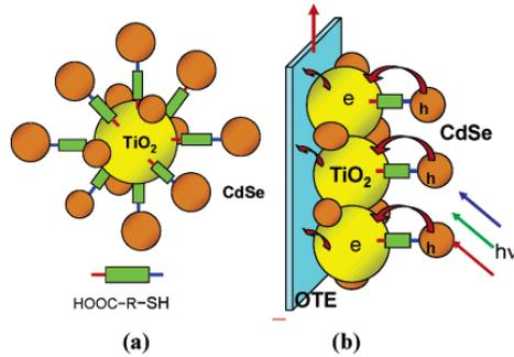
**Fig. 3: (a) Linking CdSe Quantum Dots to  $\text{TiO}_2$  Particle with Bi-functional Surface Modifier; (b) Light Harvesting Assembly Composed of  $\text{TiO}_2$  Film Functionalized with CdSe QDs on Optically Transparent Electrode (Not to Scale) <sup>[31]</sup>.**
