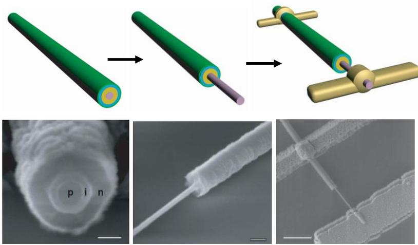
**Fig. 7. Coaxial silicon nanowire photovoltaic cell <sup>[11]</sup>:**
