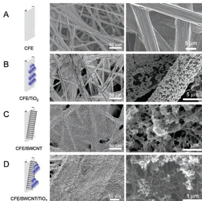
Fig. 2. SEM of a carbon fiber electrode (CFE) at different stages of modification [22]:
