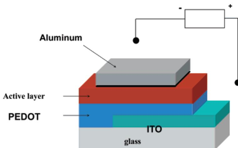
Fig. 4. Schematic device structure for polymer/fullerene bulk heterojunction solar cells. The active layer is sandwiched between two contacts: an indium-tin-oxide electrode coated with a hole transport layer PEDOT:PSS and an aluminum top electrode <sup>[44]</sup>.
