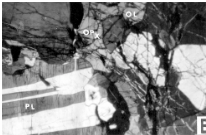
FIG. 4 – A. Cumulus plagioclase (PL) with very minor intercumulus clinopyroxene (CPx), anorthosite, Khor Fakkan area. C.N., \times 30 . B. Gabbroic cumulate showing cumulus labradorite (PL) and clinopyroxene (CPx), normal gabbro, Wadi Hatta area. C.N., \times 30 .
