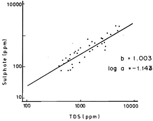
FIG. 6. Plot of *TDS* versus  $\text{SO}_4^{--}$ .
