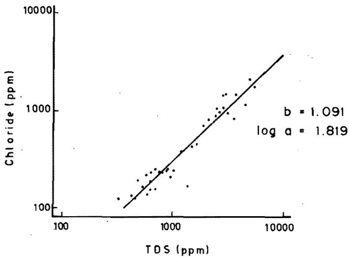
FIG. 9. Plot of *TDS* versus  $\text{Cl}^-$ .
