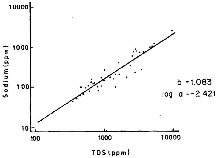
FIG. 10. Plot of *TDS* versus  $\text{Na}^+$ .
