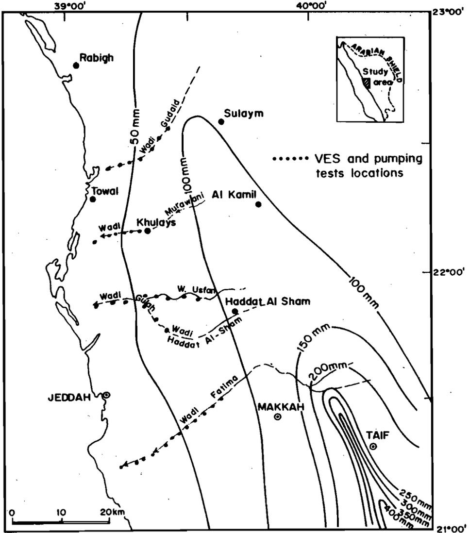
FIG. 1. Location of major wadies and average rainfall distribution over the study area, showing the locations of pumping test and VES in the study area.
