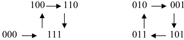
Fig. 3. The state diagram in Fig. 2 with states designated by the binary values of the 3-tuple x_1x_2x_3 .
