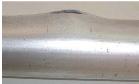
Fig. 15a: Bulging in the aluminum pipe after reaching a pressure of 300 bars (30.4 MPa).
