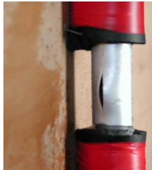
Fig. 6: The split in the extruded aluminum pipe, and the shape of the ejected water jet on the support panel.
