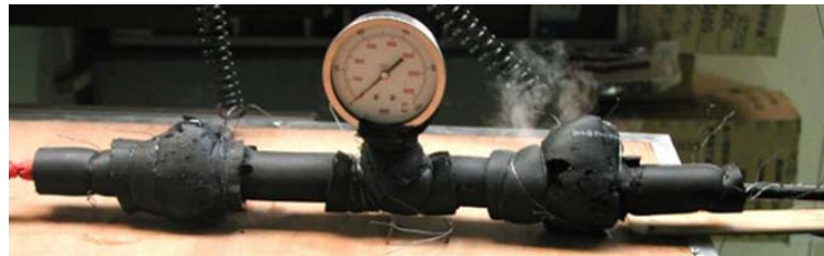
Fig. 10: Fully insulated test system with a seamless sensor pipe (above) and a dial gauge.
