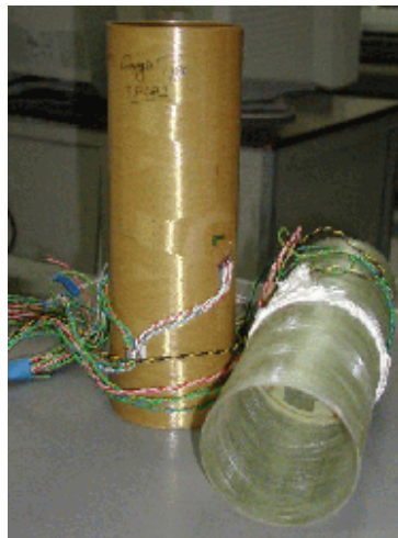
Fig. 11. Two tubes made from composite materials.
