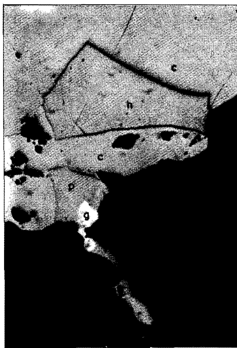
FIG. 6. Gold (g) with petzite (p) in chalcopyrite (c) containing hessite (h). Al Masani, core sample 38153, \times 200 , massive-sulfide gold-bearing mineralization type 2.
