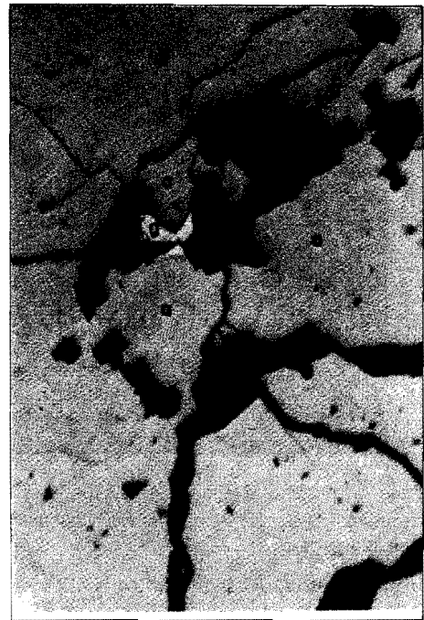
FIG. 9. Gold (g) included in fractured arsenopyrite (a). Sukhaybarat, core sample 45952, \times 500 plutonic-related gold mineralization type 4.
