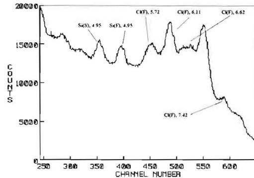
Fig. 4. Experimentally measured spectrum of prompt  $\gamma$ -rays with energies above 3 MeV from a coal sample containing 4 wt. % chlorine
