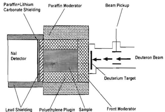
Fig. 1. Schematic of the PGNAA setup used in the study.
