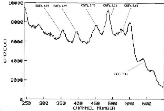
Fig. 3 Experimentally measured spectrum of prompt  $\gamma$ -rays with energies above 3 MeV from a coal sample containing 2 wt. % chlorine .
