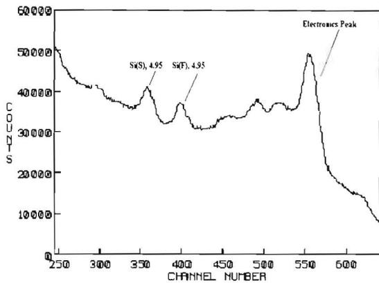
Fig. 2. Experimentally measured prompt  $\gamma$ -rays spectrum from pure coal sample with energies above 3 MeV.
