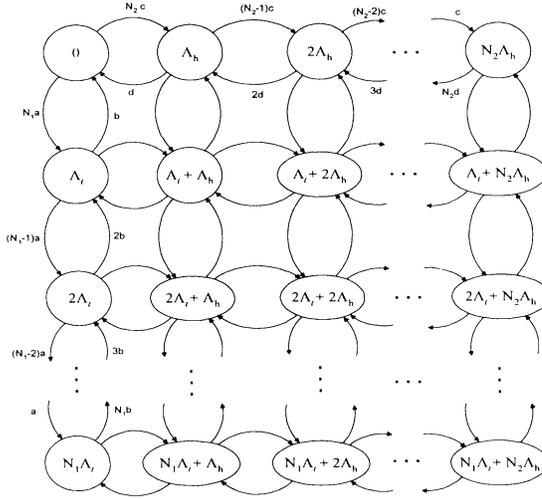
Fig. 3. State-transition-rate diagram for the aggregate source model.
