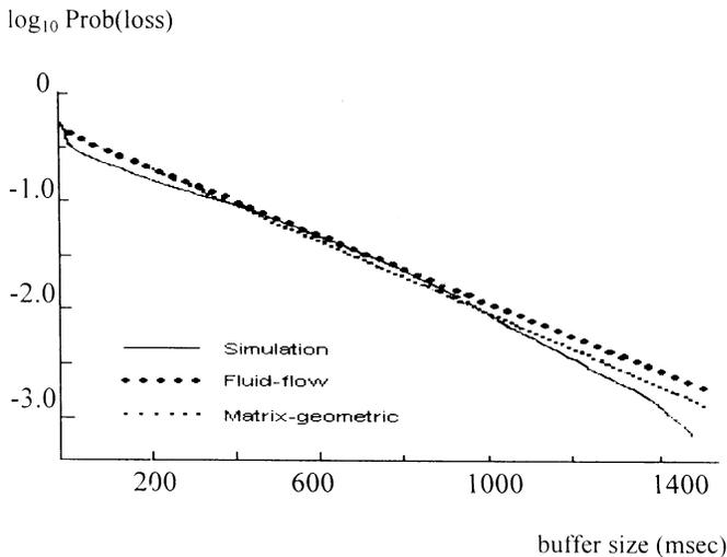
Fig. 4. Comparison to fluid-flow model and simulation.
