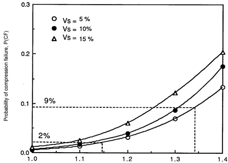
Fig. 4. Variation of the probability of compression failure with yield strength of steel at  $\rho = 0.6 \rho_b$ .
