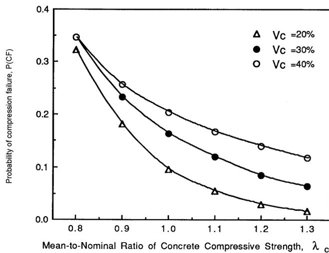
Fig. 5. Variation of the probability of compression failure with the mean-to-nominal ratio of compressive strength of concrete.
