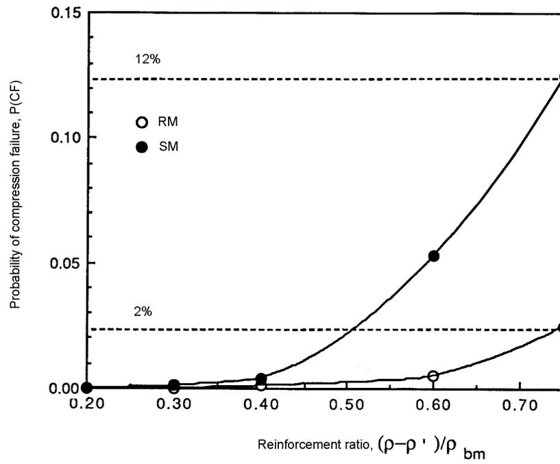
Fig. 9. Variation of the probability of compression failure with the modified reinforcement ratio for ready mixed (RM) and site mixed (SM) concretes.
