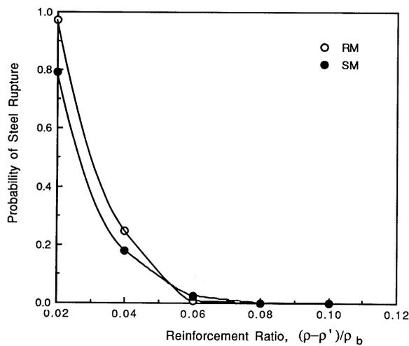
Fig. 7. Variation of the probability of steel rupture with reinforcement ratio for ready mixed (RM) and site mixed (SM) concretes.
