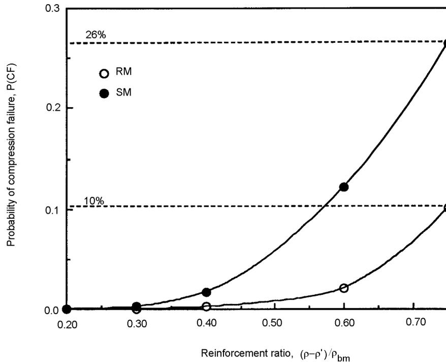
Fig. 10. Variation of the probability of compression failure with the modified reinforcement ratio under earthquake rate of loading for ready mixed (RM) and site mixed (SM) concretes.
