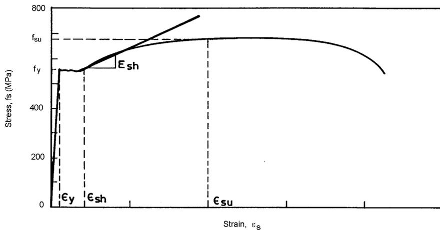
Fig. 2. Typical stress-strain relationship for (HADEED) steel.
