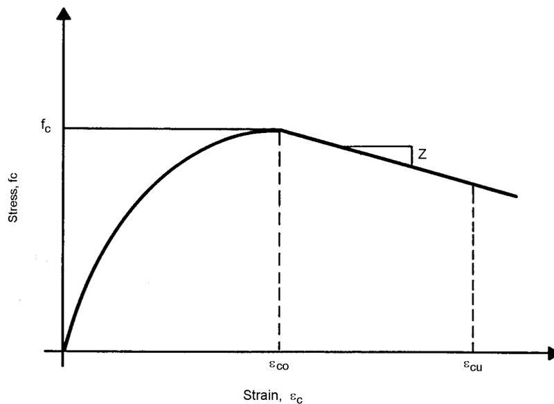
Fig. 1. Stress-strain relationship for concrete.
