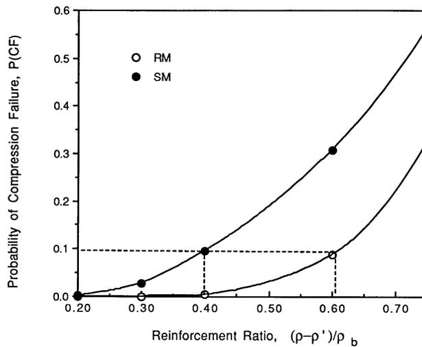
Fig. 6. Variation of the probability of compression failure with the reinforcement ratio for ready mixed (RM) and site mixed (SM) concretes.
