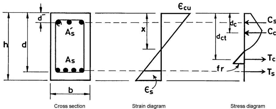
Fig. 3. Stress and strain distributions for RC section.
