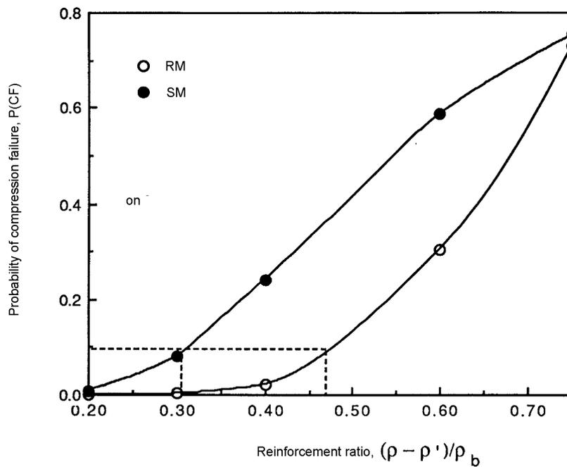
Fig. 8. Variation of the probability of compression failure with reinforcement ratio at earthquake rate of loading for ready mixed (RN) and site mixed (SM) concretes.
