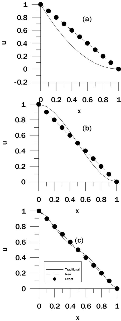
Fig. 3. Concentration profiles for the zero-order reaction with  $k=1$ ,  $Pe=1000$  for (a) $N=1$ ,  $NN=2$ , (b) $N=2$ ,  $NN=4$ , (c) $N=4$ ,  $NN=8$ .
