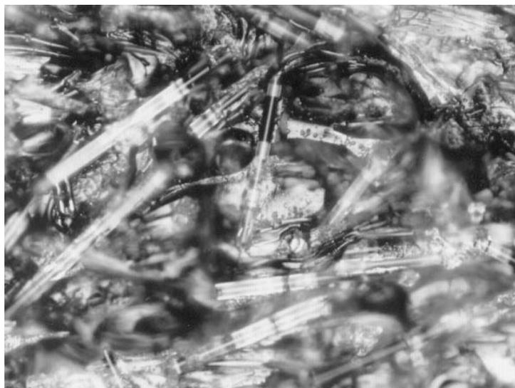
**Fig. 3. Optical image of the PEI's surface after chromic acid solution treatment. Glass fibers are clearly indicated in the image. At 200x magnification.**
