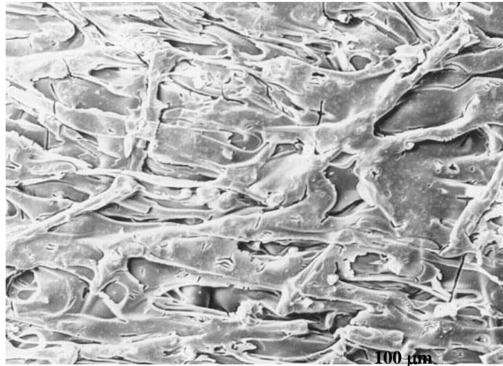
Fig. 4. Scanning electron photomicrograph of the PEI surface after glass etching treatment.
