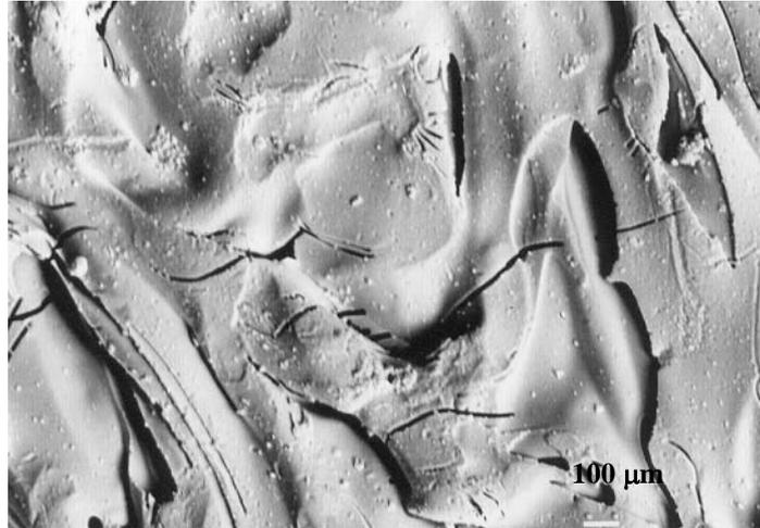
**Fig. 6. Scanning electron photomicrograph of electroless copper deposited on treated PEI surface.**
