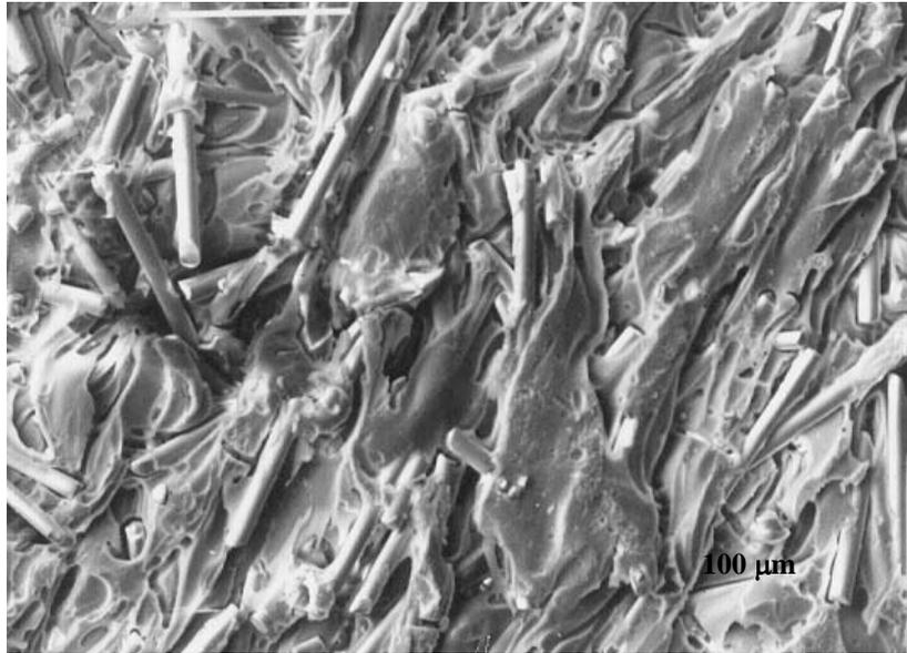
Fig. 2. Scanning electron micrograph of the PEI surface after chromic acid solution treatment.
