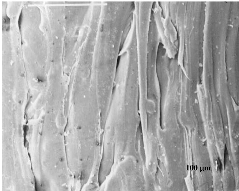
Fig. 1. Scanning electron micrograph of the initial PEI surface.
