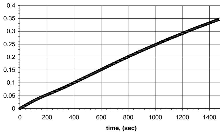
Fig. 5. Quartz crystal microbalance result for copper electroless solution.
