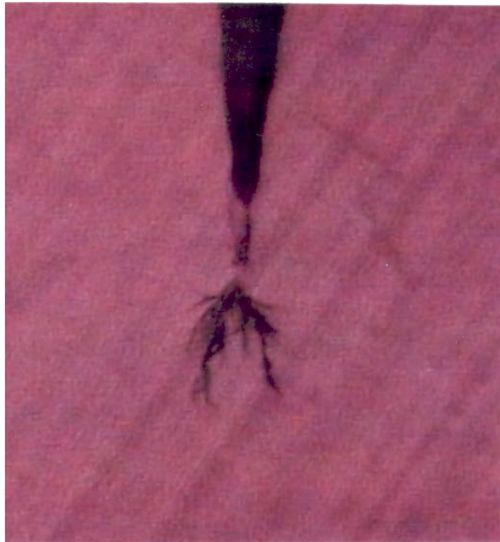
Fig. 6. Propagation of electrical tree from the tip of water tree due to \text{AgNO}_3 for cable with outer semiconducting screen. Tree length 426 \mu\text{m} .
