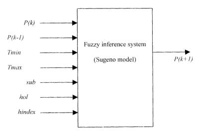
Fig. 7. A general structure of the fuzzy neural forecasting model.
