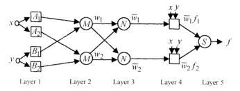
Fig. 5. Equivalent ANFIS architecture [11].
