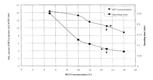
Fig. 5. Minimum amount required and spending time of HCl in different concentrations to dissolve 1g of CaCO<sub>3</sub>.
