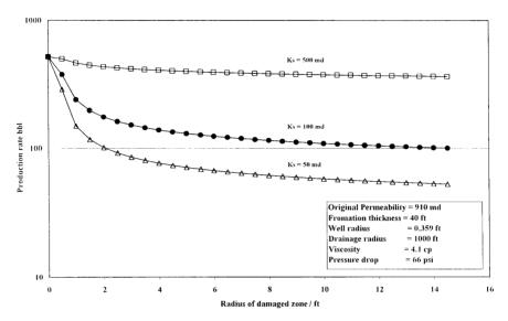
Fig. 1. Influence of the radius of damaged zone on the well productivity.
