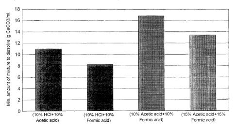
Fig. 7. Comparison between different acid mixtures.
