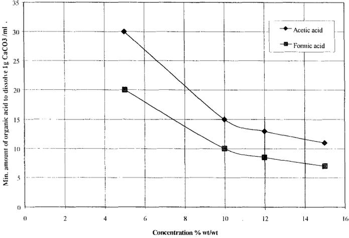
Fig. 6. Minimum amount of organic acids required to dissolve 1g of CaCO<sub>3</sub>.
