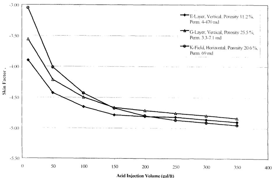
Fig. 9. Skin factor vs. acid injection volume after well completion for vertical and horizontal wells.
