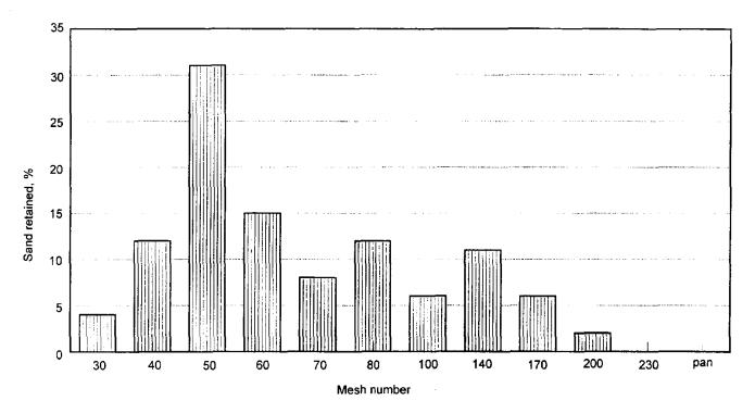
Fig. 1. Granulometric analysis of friable sand used.
