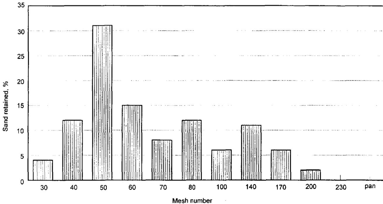
Fig. 1. Granulometric analysis of friable sand used.
