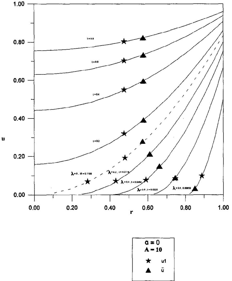
Fig. 4. Temperature profile for transient heat conduction.
