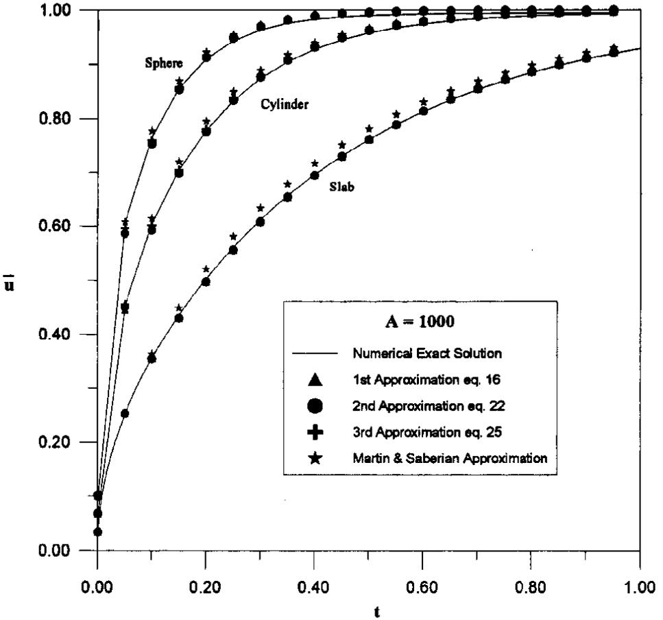
Fig. 2. Comparison of average temperatures for different shapes.
