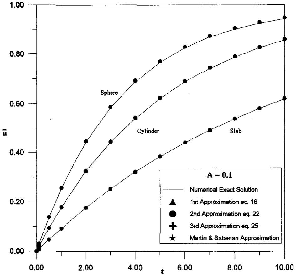
Fig. 3. Comparison of average temperatures for different shapes.
