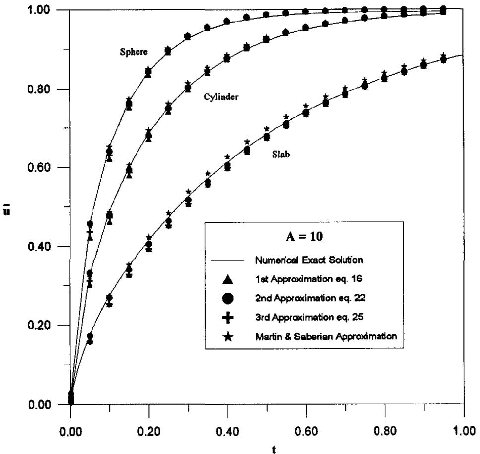
**Fig. 1. Comparison of average temperatures for different shapes.**
