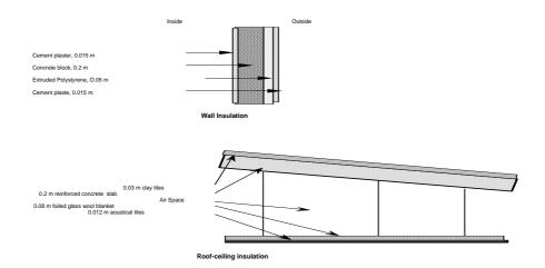
Fig. 2. Walls and roof ceiling after applying thermal insulation.
