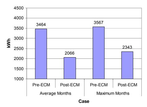
Fig. 6. A/C Electrical consumptions due to building envelope.
