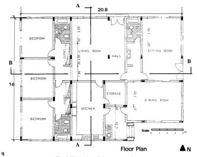
Fig. 4. Floor plan of the one-story house.
