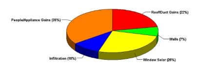
Fig. 1. Annual cooling load components [9].
