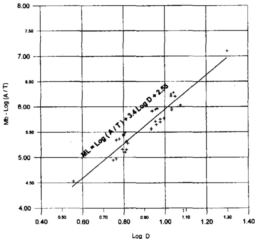
Fig. 3. Plotted data used in determining the adopted local magnitude scale (ML). The vertical axis represents the difference values between the body-wave magnitude ( $mb$ ) and the corresponding logarithm of amplitudes ( $A/T$ ) in micrometer. Abscissa is the logarithm of the corresponding epicentral distance ( $D$ ) in degrees.
