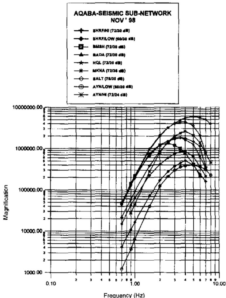
Fig. 2. Analog system response curves for eight short-period seismic stations of the Aqabah sub-network in NW Saudi Arabia.
