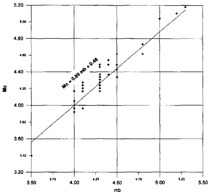
Fig. 6. Plottings of corresponding calculated coda magnitude ( $M_c$ ) and observed body-wave magnitude ( $m_b$ ) values used in determining the empirical relation. Vertical axis is  $M_c$  and horizontal axis is  $m_b$ .
