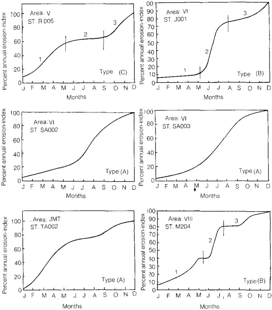
Fig. 2. Rainfall erosion-index distribution curves for various regions in the Kingdom.
