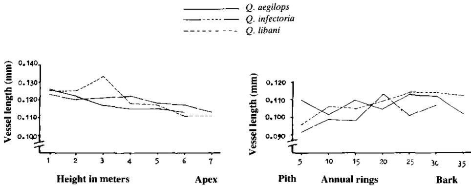
Fig. 1. Relationship of vessel length (mm) and coded tree height and rings classes of Iraqi oak species.
