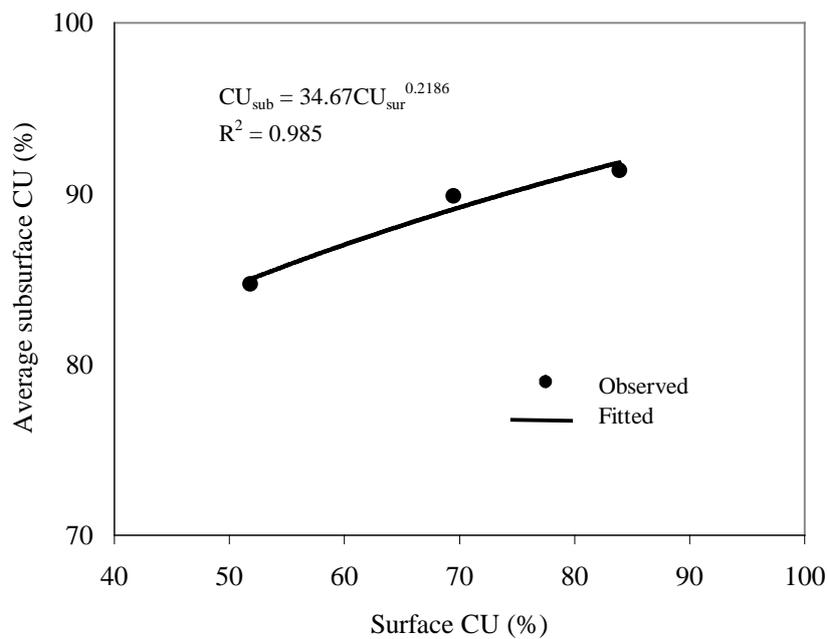
Fig. 4. Average subsurface vs. surface CU normal to pivot.
