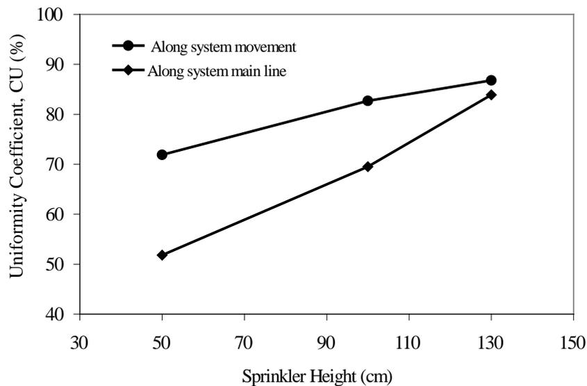
Fig. 2. Relationship between surface CU and sprinkler height.
