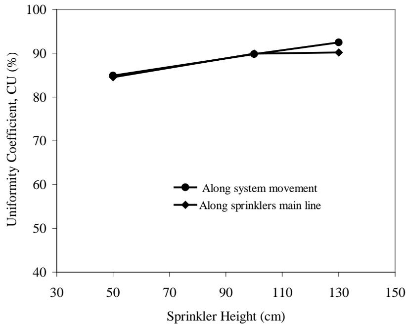
**Fig. 3. Relationship between subsurface CU and sprinkler height.**
