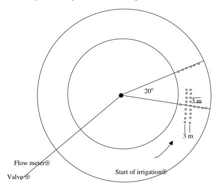
Fig. 1. Layout of the field experiment.
