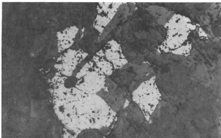
Plate 1. WSHL — Photomicrograph showing exsolution lamellae of ilmenite in magnetite. X 32.
