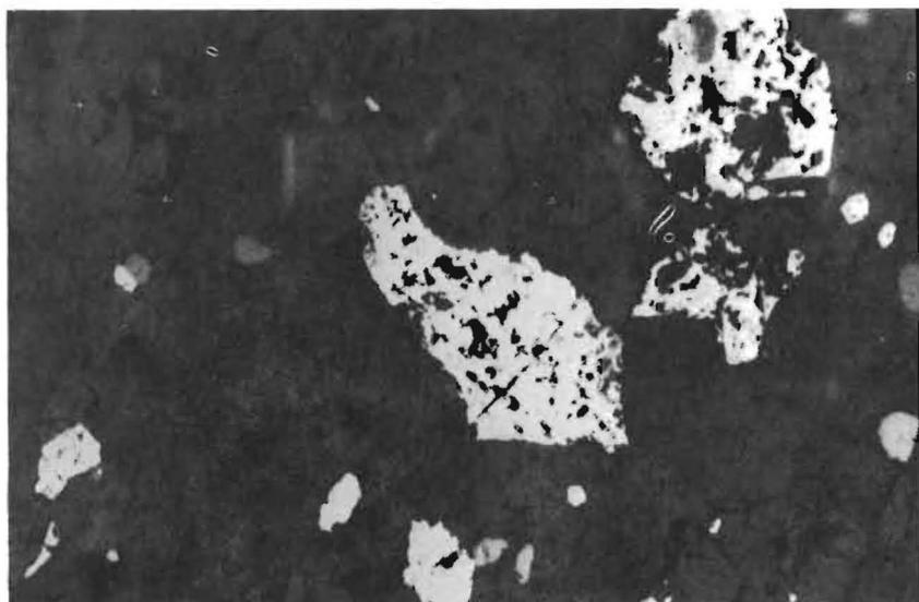
**Plate 5. WSH<sub>3</sub> — Large discrete grains of Pyrrhotite (clear grey) in silicates. X 32.**
