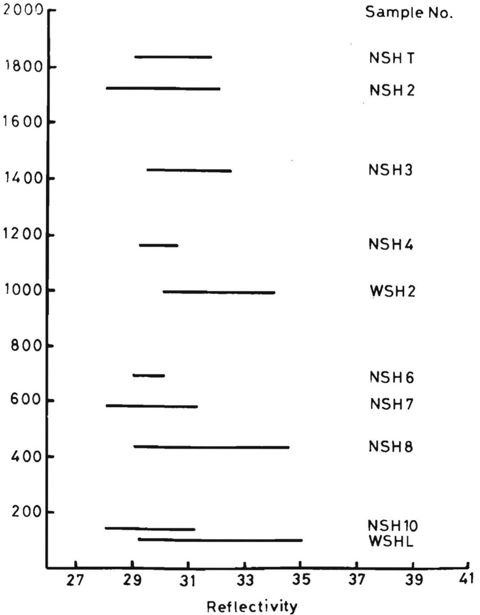
Fig. 4. Variation of reflectivity in Pyrrhotite with the structural height of the intrusion.
