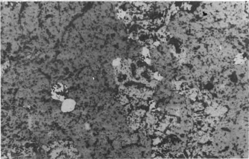
**Plate 4. NSH<sub>2</sub> — Small droplets of sulphides, mainly pyrrhotite in silicates. X 32.**
